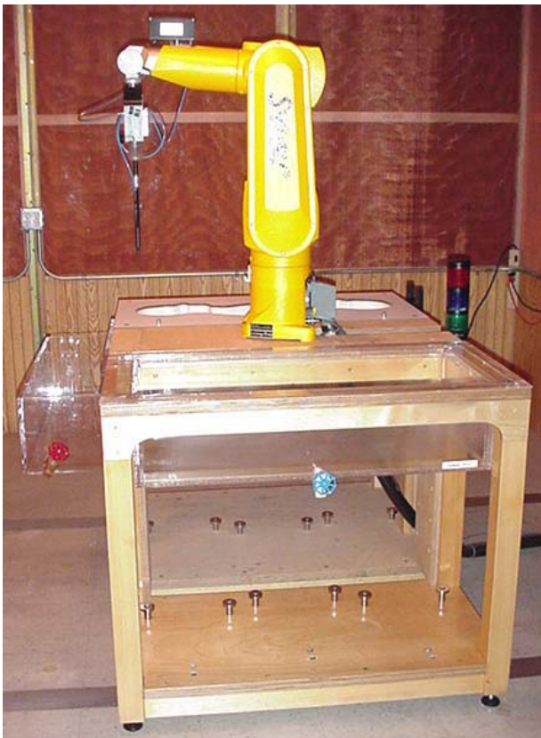
DASY4 SAR Measurement System with validation phantom
