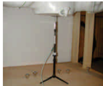
Figure 12.1 Dipole Validation Test Setup
