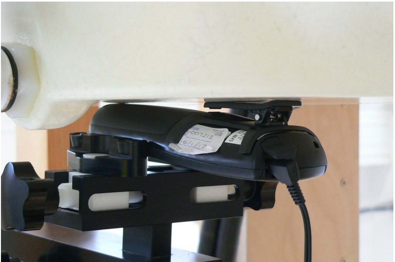
Fig. 21: Body worn configuration for D160, position 2, display towards the ground, headset and clip attached, 0 mm distance.
