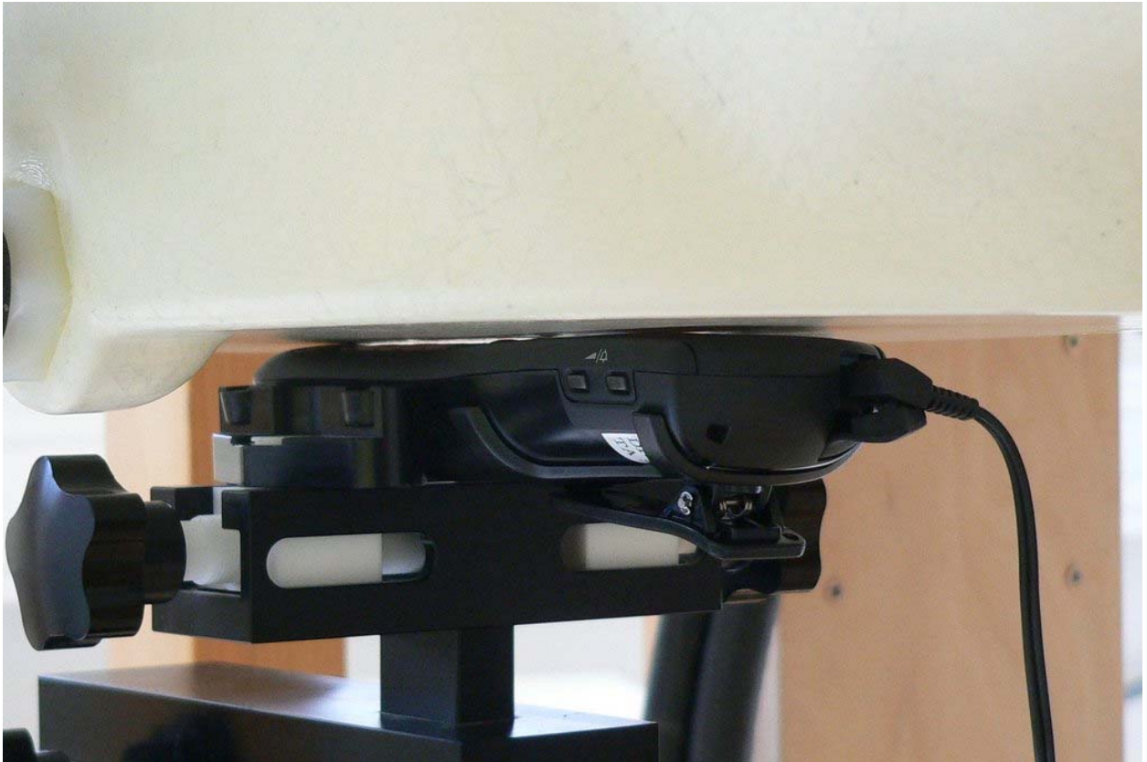
Fig. 20: Body worn configuration for D160, position 1, display towards the phantom, headset and clip attached, 0 mm distance.
