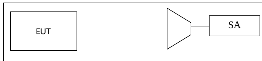
Figure A-1. Test Instrument & Measurement Setup
