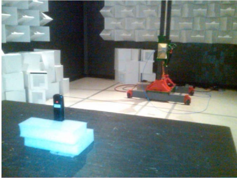
Photo 6 Test Setup – Radiated Emissions
