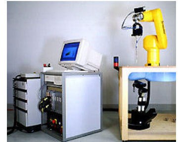
Fig. 1 SAR Test Setup
