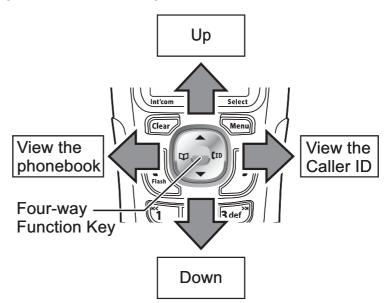
To use this four-way key, place your thumb over the key on the handset and move to the four positions to get the feel of how it moves and operates.
