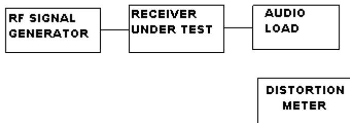
**TEST PROCEDURE:** The reference sensitivity was measured in accordance with TIA/EIA-603;
