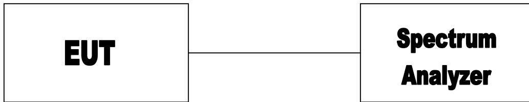
All measurements resulted in readings less than -80 dBm or less than .01 nanoWatts.
