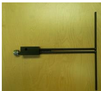
Figure 1 – MVG COMOSAR Validation Dipole
