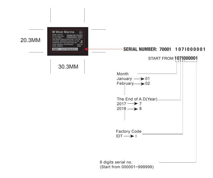
Rating Label for Unit PN:300208968-00001-10 Size:30.3x20.3mm(+/-0.2MM) Material:25# ALUMINIUM LABEL(哑银箔Recycle) Finish:Finish:W/PP Coating Color:sliver text on Black background
