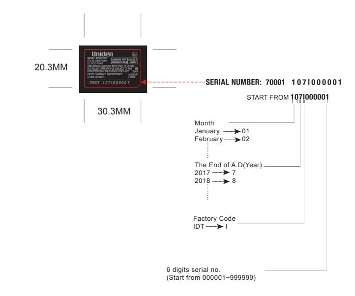
Rating Label for Unit PN:300208968-00001-10 Size:30.3x20.3mm(+/-0.2MM) Material:哑银箔Recycle(Th'k0.2mm sliver paper) Finish:Finish:W/PP Coating Color:sliver text on Black background
