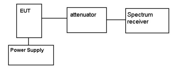
**METHOD OF MEASUREMENT:** The procedure used was EIA/TIA-382-A.
