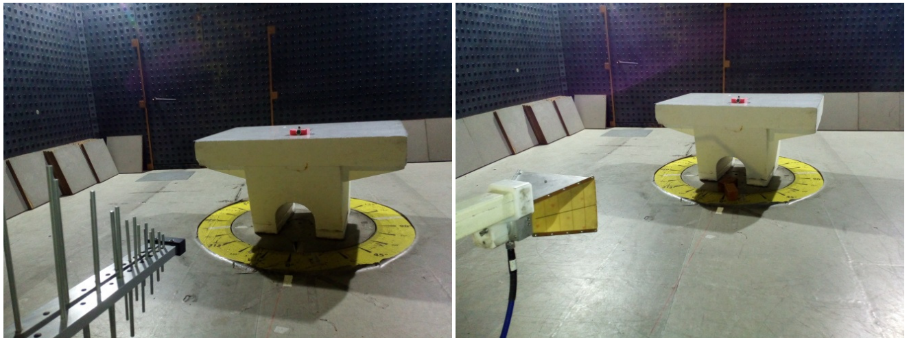
Photograph 8.1.1 Setup for radiated emission measurements
