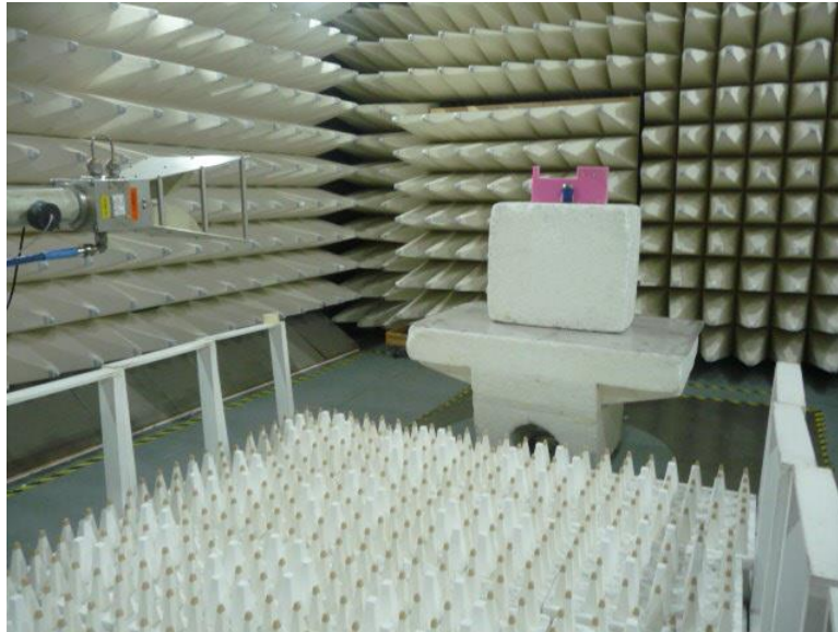
Photograph No.3 Setup for carrier and spurious emission field strength measurements in the anechoic chamber in 1000 – 18000 MHz range
