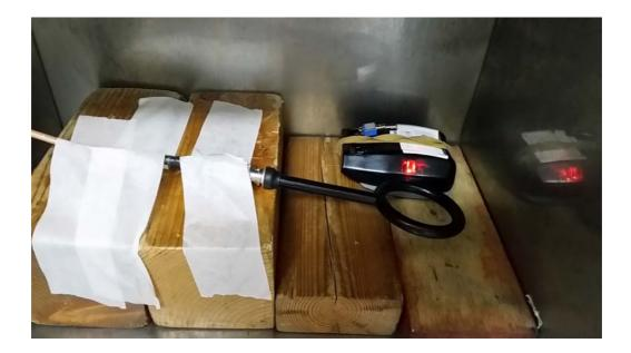
Photograph No.5 Setup for occupied bandwidth measurements
