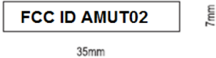
HR-TAG-LD tag, label with FCC ID AMUT02 location
