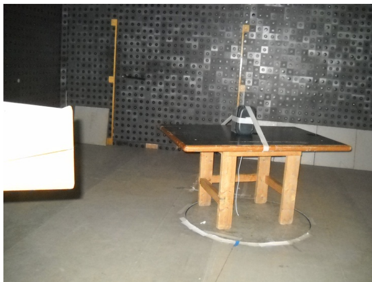
Photograph 8.1.2 Setup for radiated emission measurements
