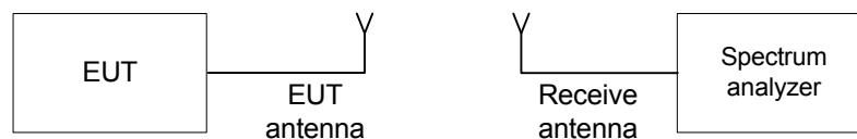
Figure 7.4.1 Occupied bandwidth test setup
