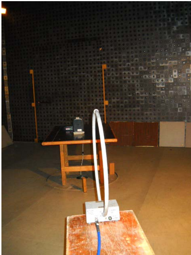
Photograph No.1 Setup for spurious emission field strength measurements in the anechoic chamber below 30 MHz
