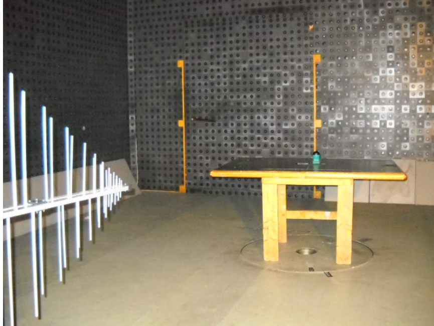
Photograph No.2 Setup for carrier and spurious emission field strength measurements in the anechoic chamber in 30 – 1000 MHz range
