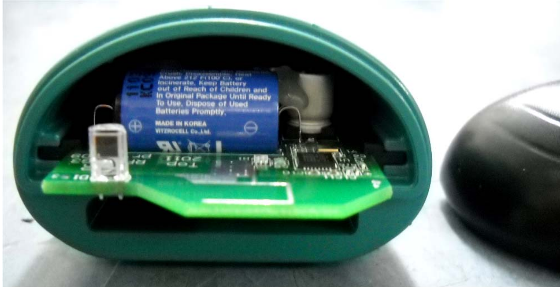
Photograph No.1 H-TAG-LD activity based tag internal view
