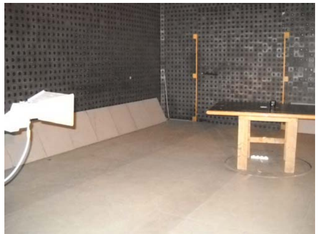
Photograph 8.1.1 Setup for radiated emission measurements
