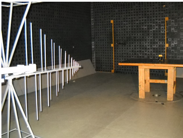
Photograph 8.1.1 Setup for radiated emission measurements
