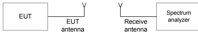
Figure 7.4.1 Occupied bandwidth test setup
