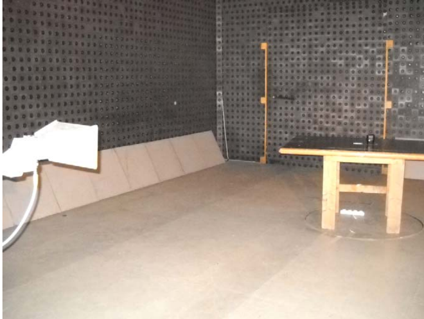
Photograph No.3 Setup for spurious emission field strength and OBW measurements in the anechoic chamber in 1 - 18 GHz range
