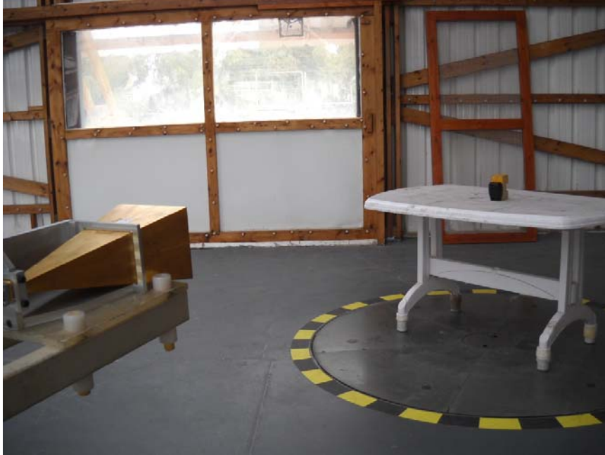
Photograph No.4 Setup for spurious emission field strength measurements at the OATS in 18 - 25 GHz range
