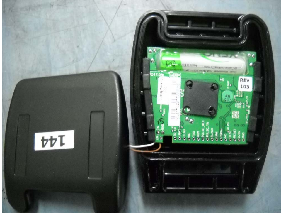
Photograph No.1 HR-TAG-LD activity&rumination based tag internal view
