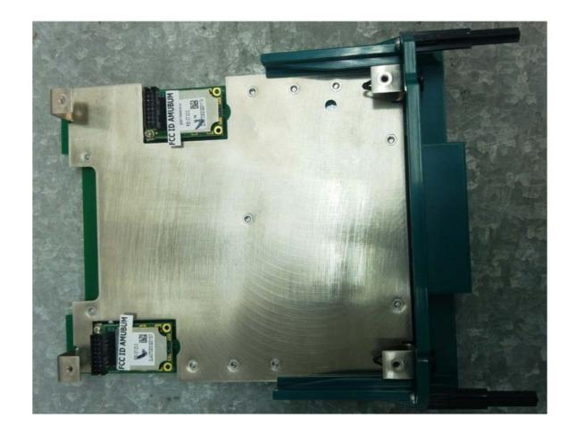
Photograph No.4 LD module with internal antenna without shield
