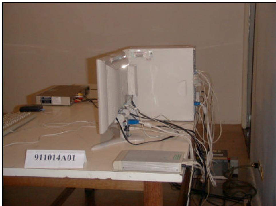
RADIATED EMISSION TEST (for Mode 1)
