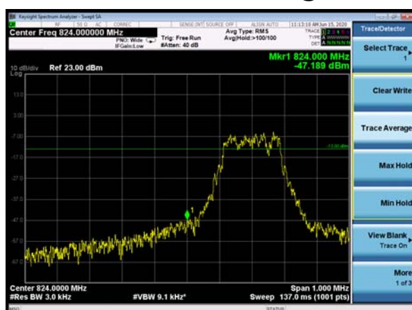
NB-IOT Band 5 QPSK 15kHz 12@0 CH-Low
