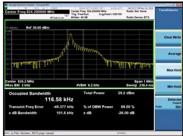
NB-IOT Band 5 BPSK 15kHz 1@0 CH-Middle
