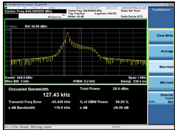
NB-IOT Band 5 BPSK 15kHz 1@0 CH-High
