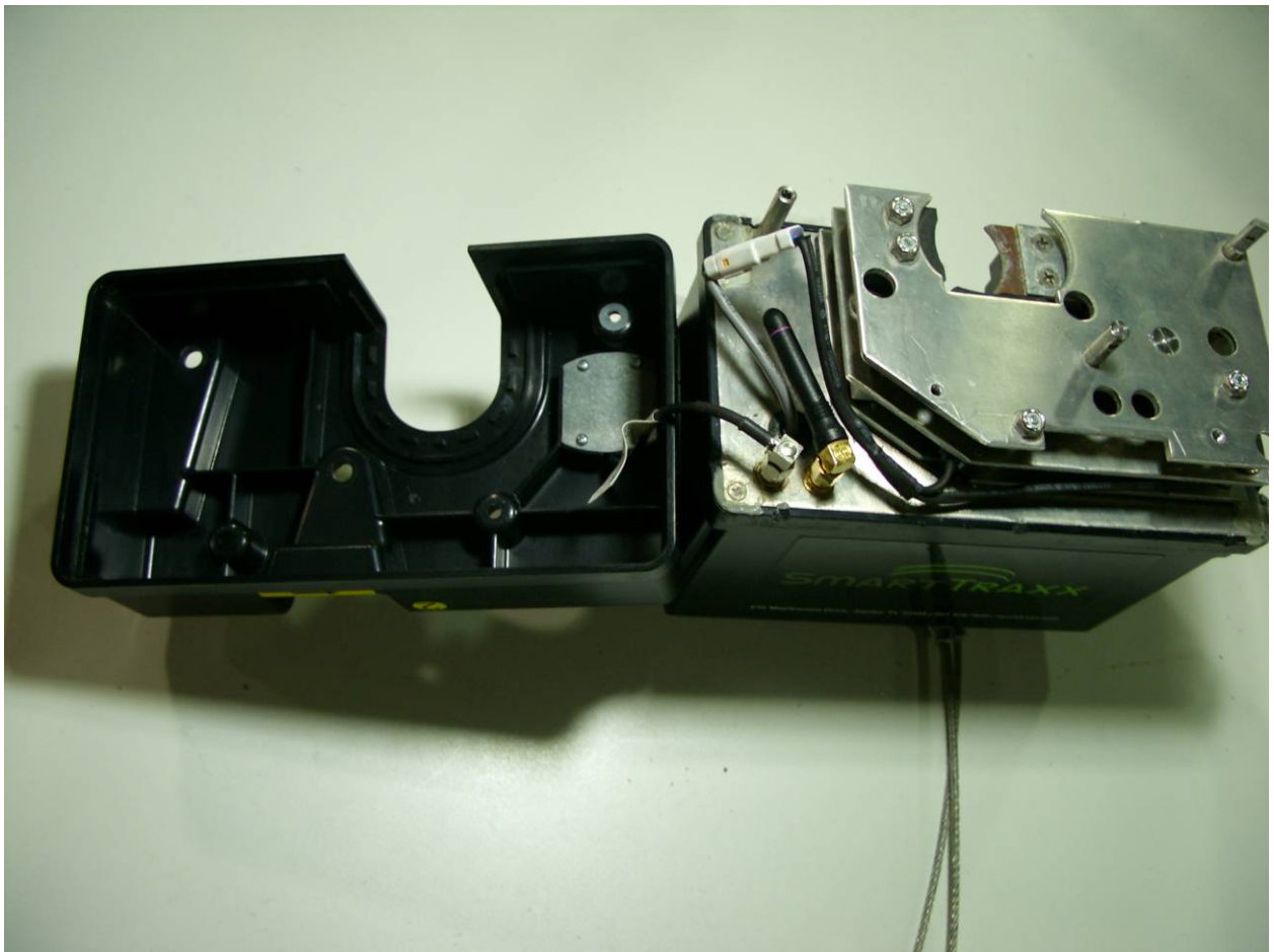
Figure 8: Internal View (showing GPS and Zigbee Antennas)
