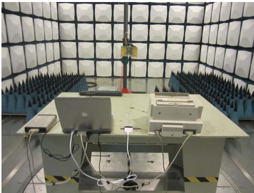
Radiated Emission – Rear View (Above 1GHz Distance 1.5m)
