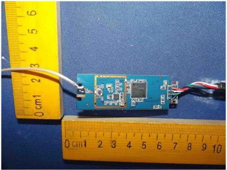
Figure 11 PCB of The EUT-Back View
