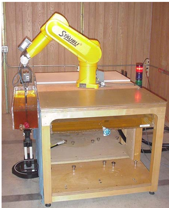
DASY4 SAR Measurement System with Side Planar Phantom
