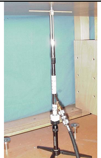
SPEAG 835 MHz Validation Dipole Setup
