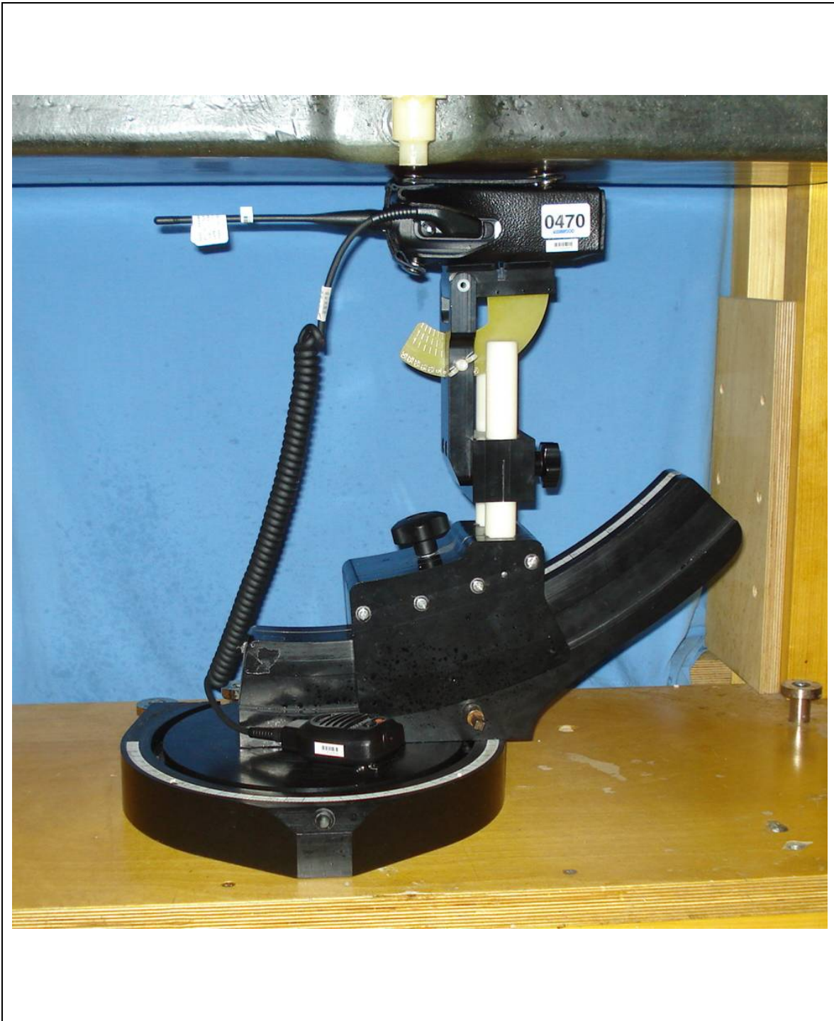
Body-worn SAR Configuration Test Setup with Leather Case
