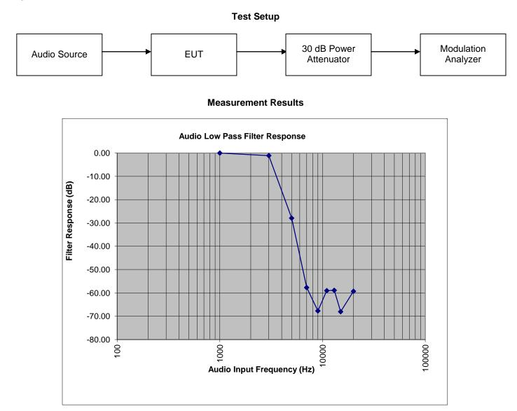
This unit is a digital radio and the roll-off for the filter is very linear in the operational band and sharp out of band.
