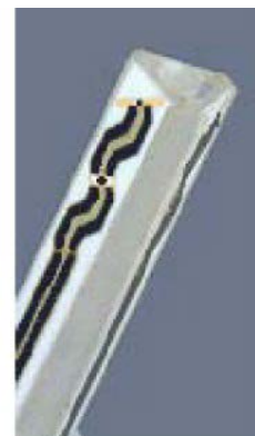
Figure 2.3 Probe Thick-Film Technique
