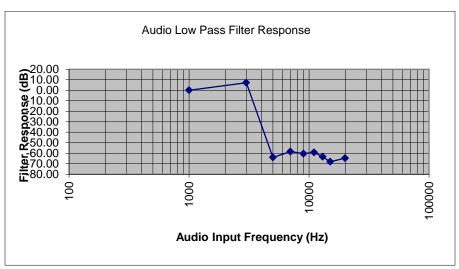
This unit is a digital radio and the roll-off for the filter is very linear in the operational band and sharp out of band.
