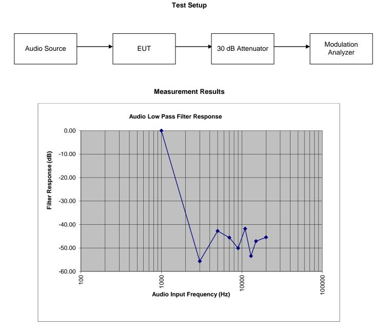
This unit is a digital radio and the roll-off for the filter is very linear in the operational band and sharp out of band.
