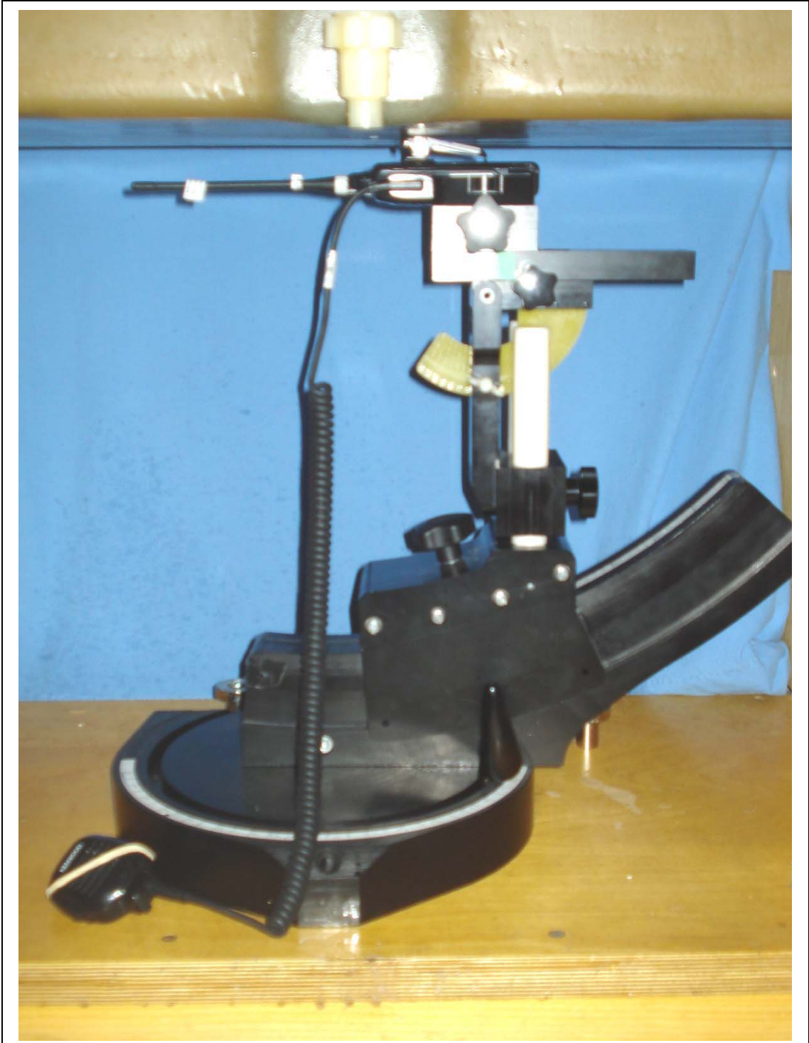
Body-worn Test Setup Configuration DUT with Belt-Clip Body-worn Accessory (P/N: J29-0751-05) & Speaker-Mic Audio Accessory (P/N: KMC-45)
