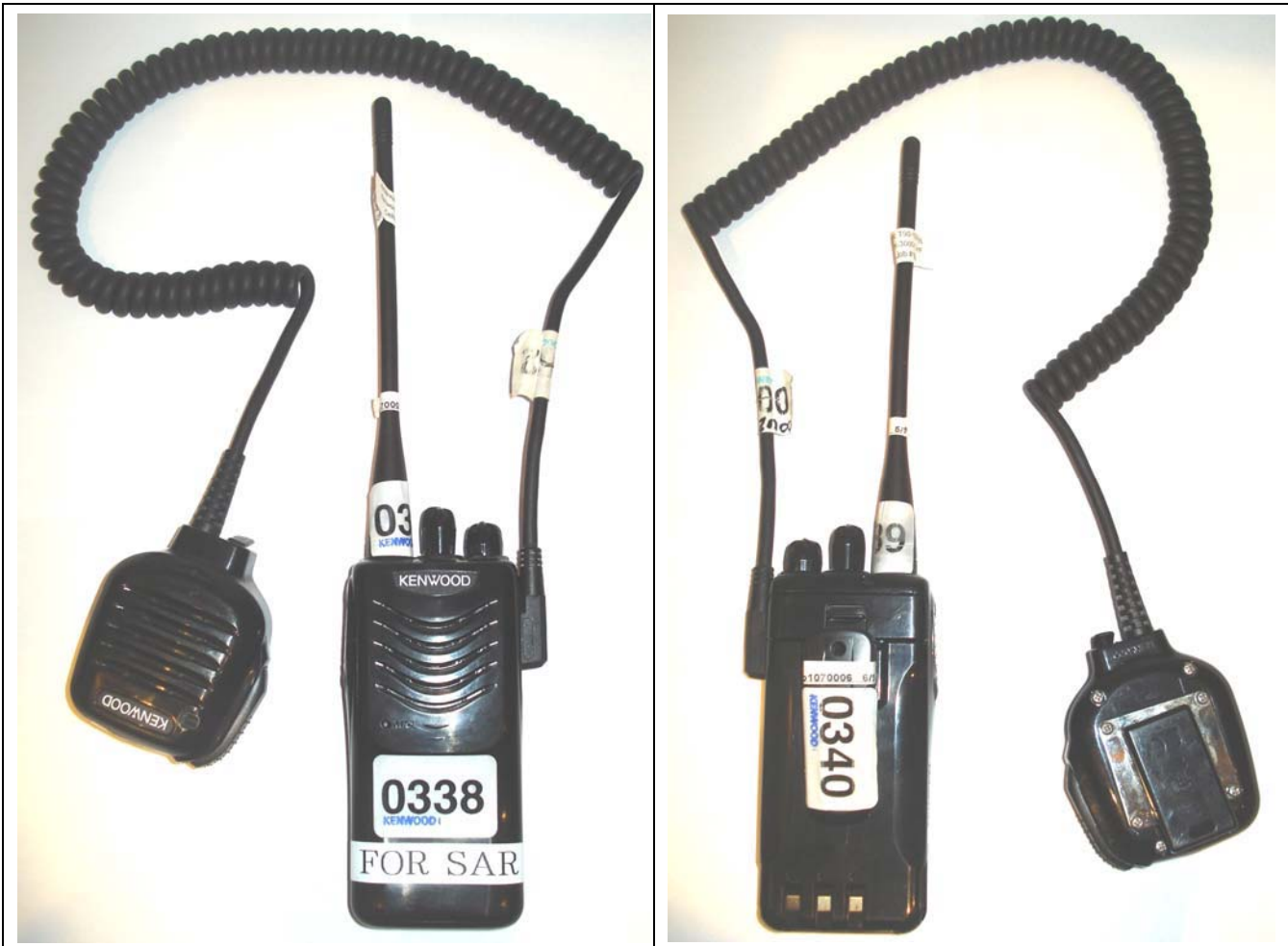
Front of DUT and Speaker-Microphone (P/N: KMC-45)
