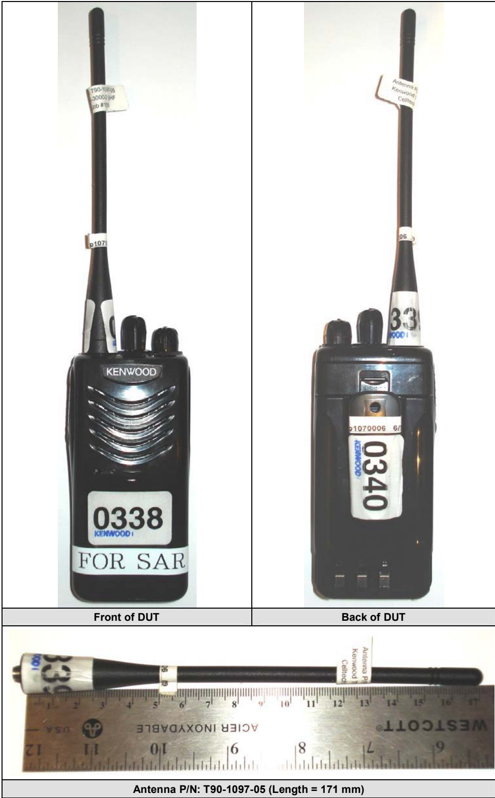
Antenna P/N: T90-1097-05 (Length = 171 mm)
