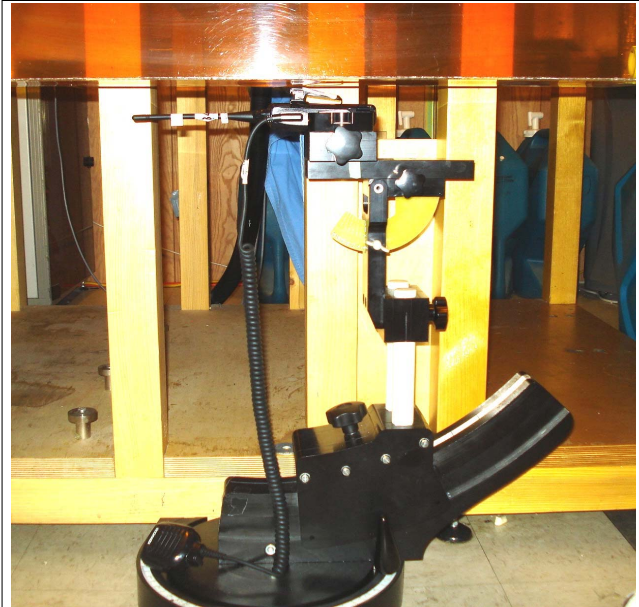
Body-worn Test Setup Configuration DUT with Belt-Clip Body-worn Accessory (P/N: J29-0751-05) & Speaker-Microphone Audio Accessory (P/N: KMC-45)
