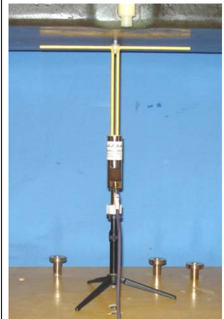
SPEAG 450 MHz Validation Dipole Setup
