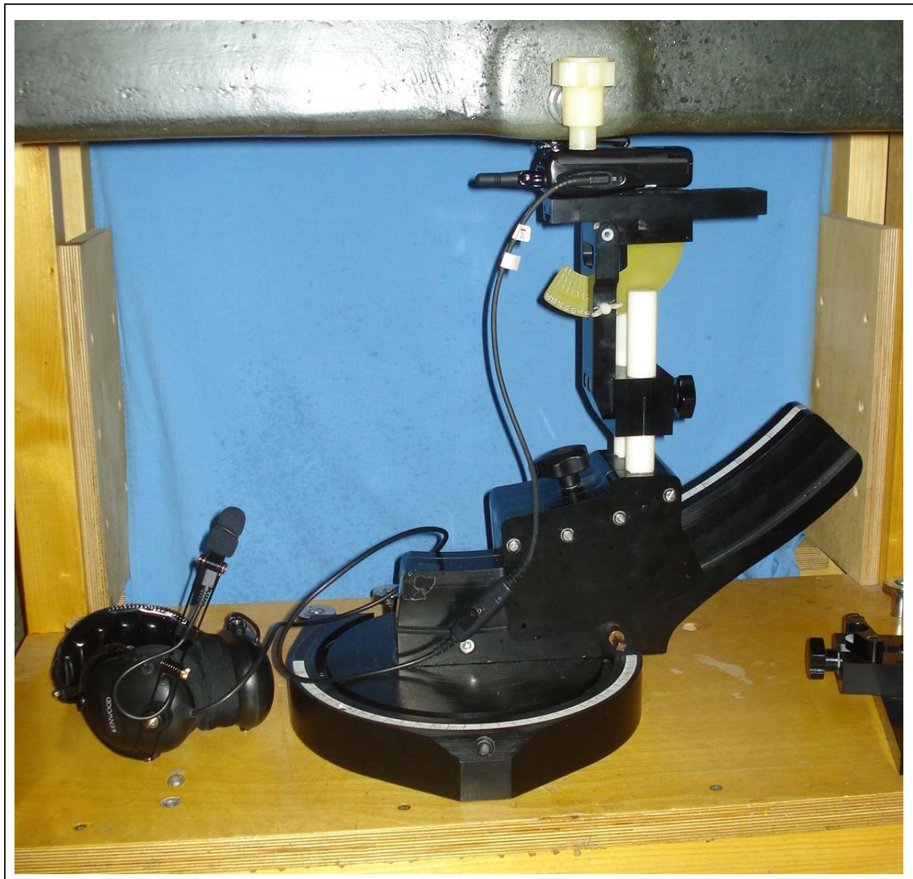
Body-worn SAR Configuration - Antenna 8, Battery a, Audio G3b
