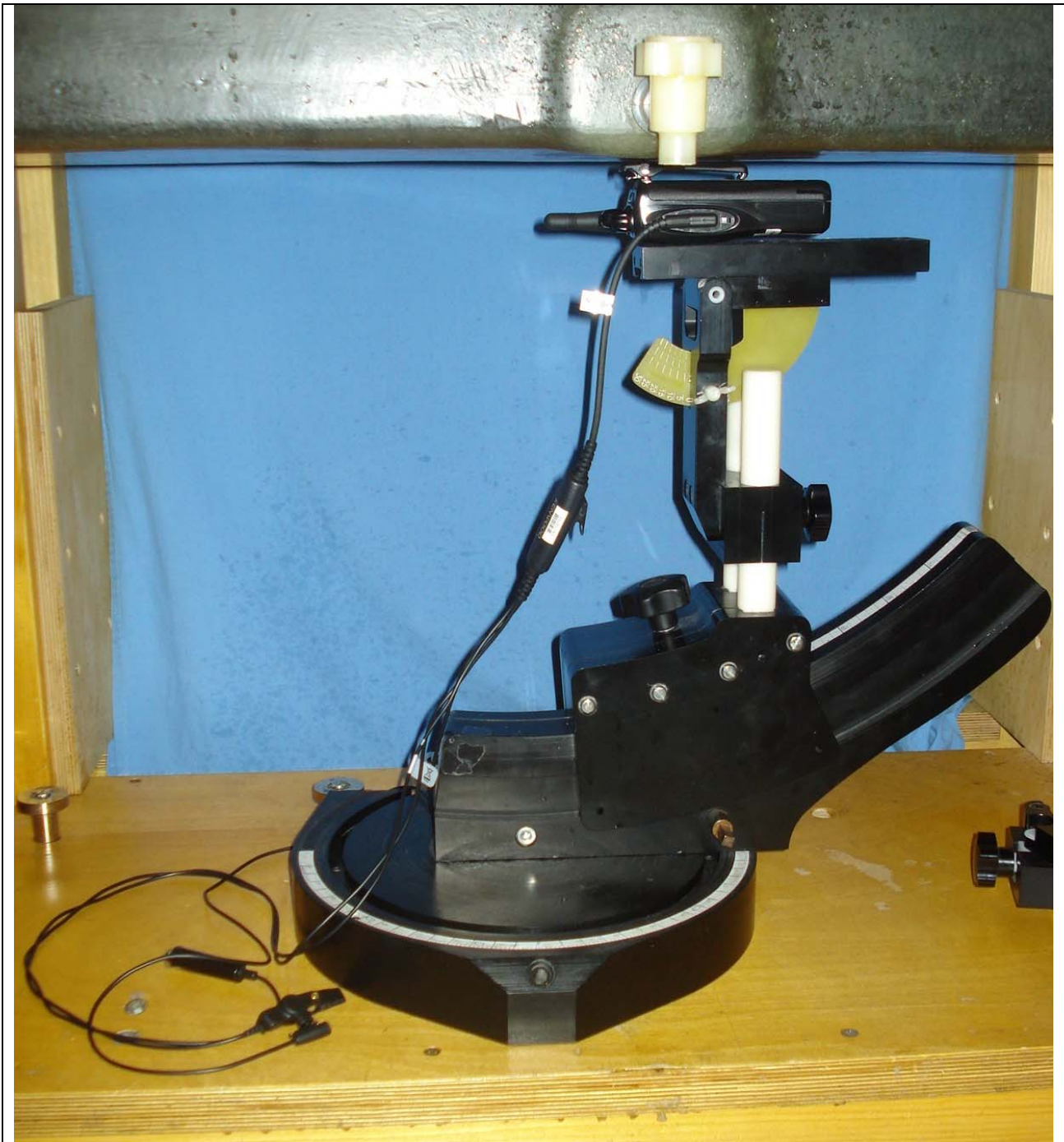
Body-worn SAR Configuration - Antenna 8, Battery a, Audio G5b
