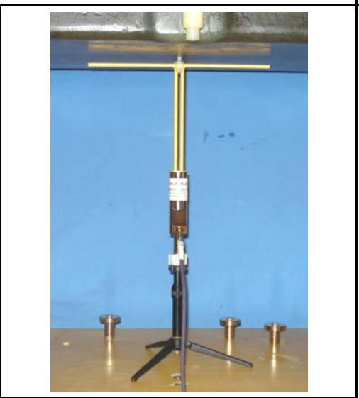
System Performance Check Measurement Setup (IEEE Standard 1528-2003) SPEAG 450 MHz Validation Dipole Setup
