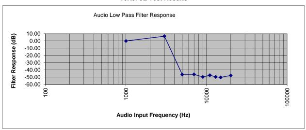
This unit is a digital radio and the roll-off for the filter is very linear in the operational band and sharp out of band.
