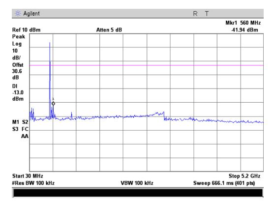
511.95 MHz Conducted Emissions Test Plots
