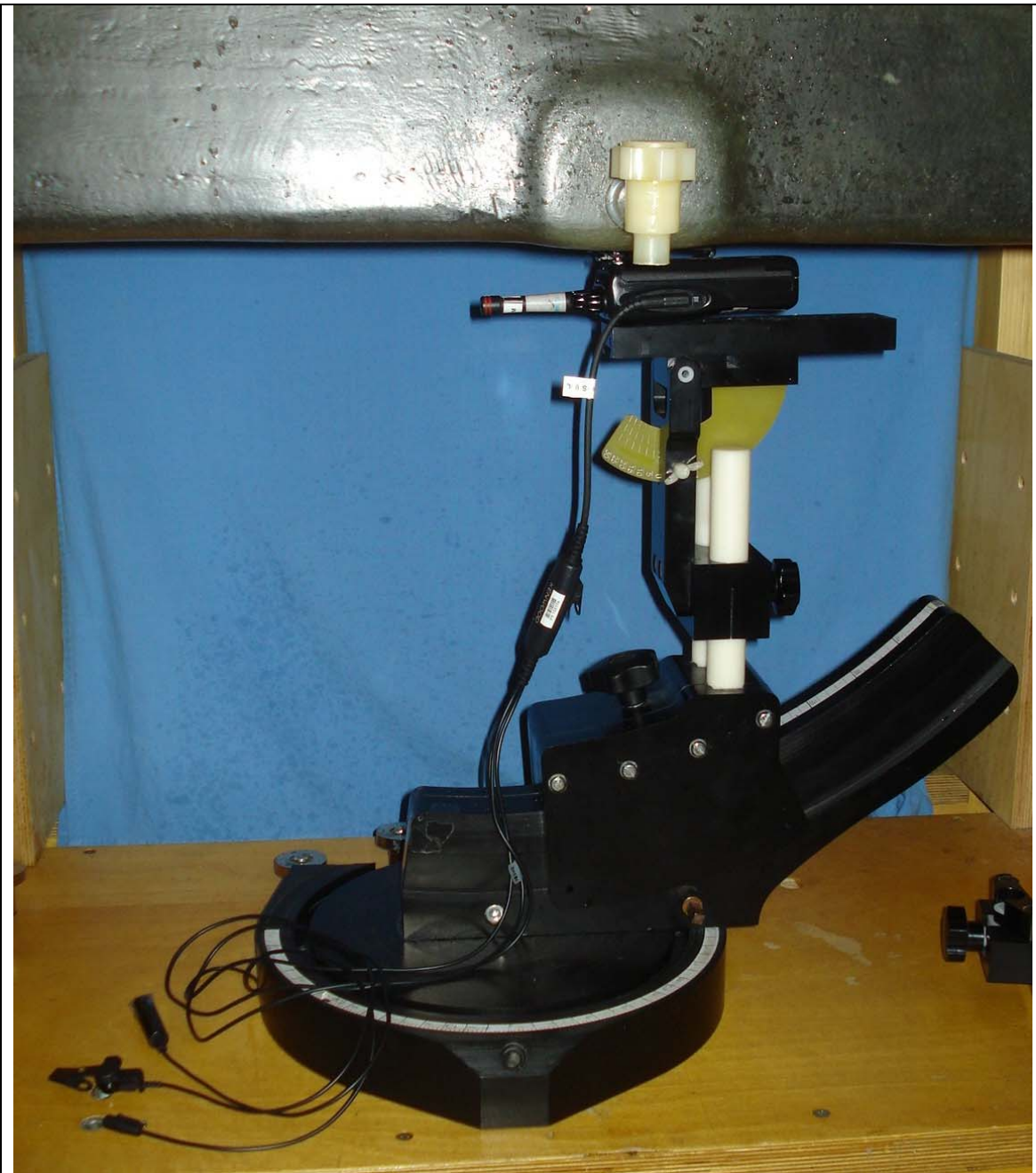
Body-worn SAR Configuration - Antenna 1, Battery a, Audio G5b
