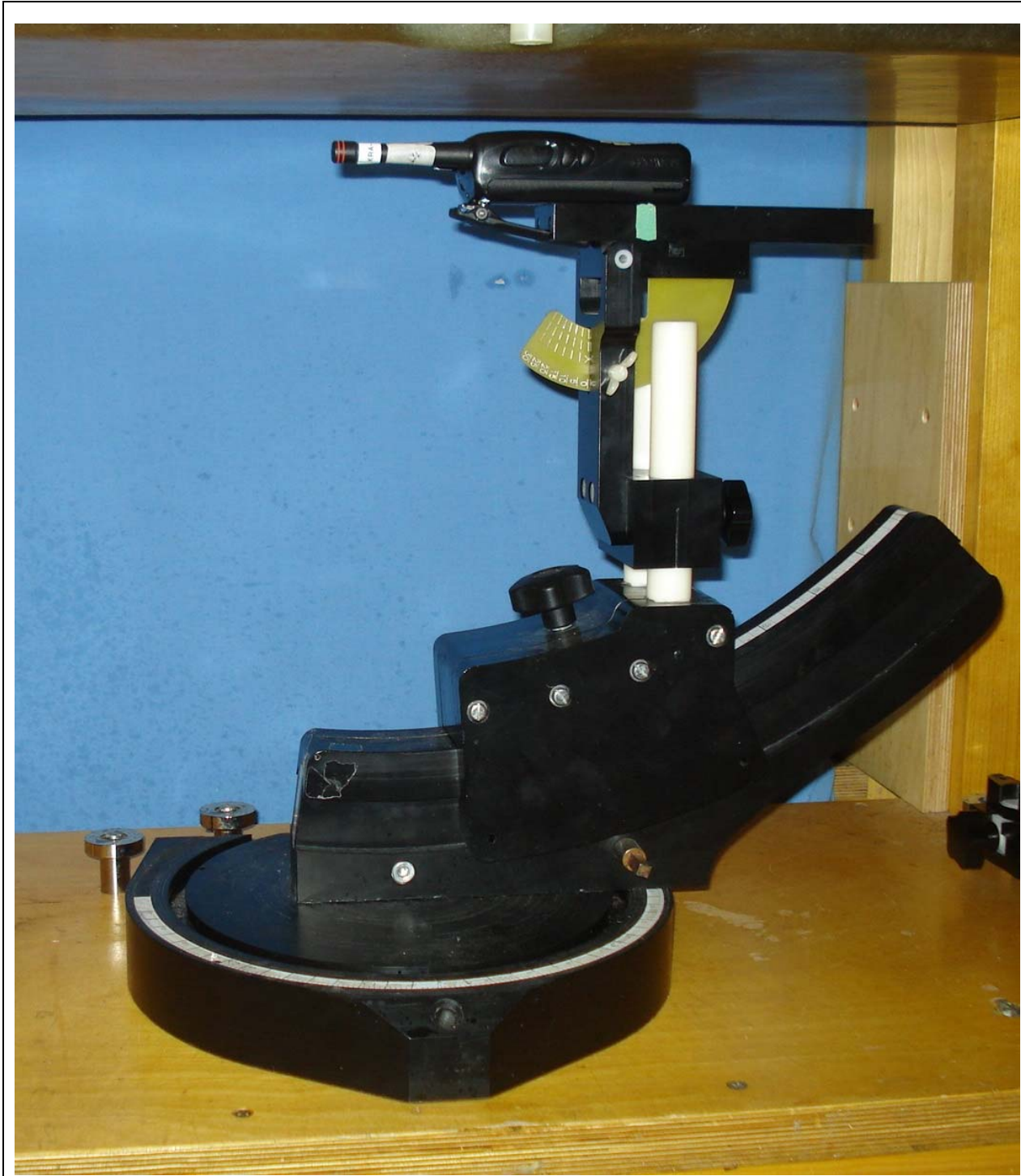
Face-held SAR Configuration Test Setup
