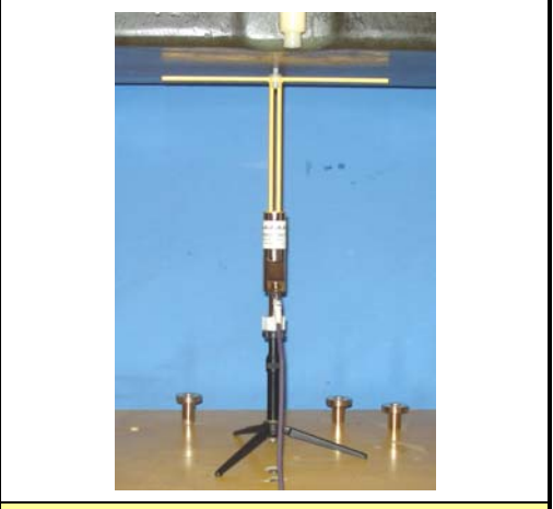
System Performance Check Measurement Setup (IEEE Standard 1528-2003) SPEAG 450 MHz Validation Dipole Setup
