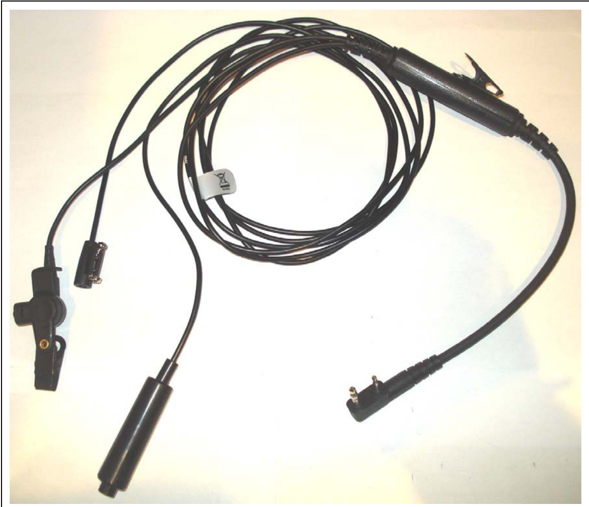
3-Wire Lapel Microphone w/ Earpiece (P/N: KHS-9BL)
