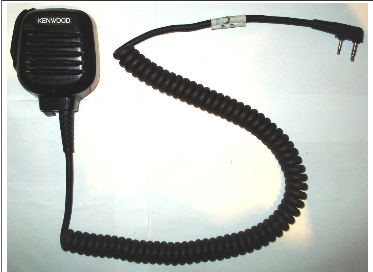
Heavy Duty Speaker-Microphone (P/N: KMC-45)
