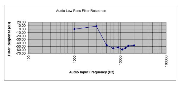
This unit is a digital radio and the roll-off for the filter is very linear in the operational band and sharp out of band.
