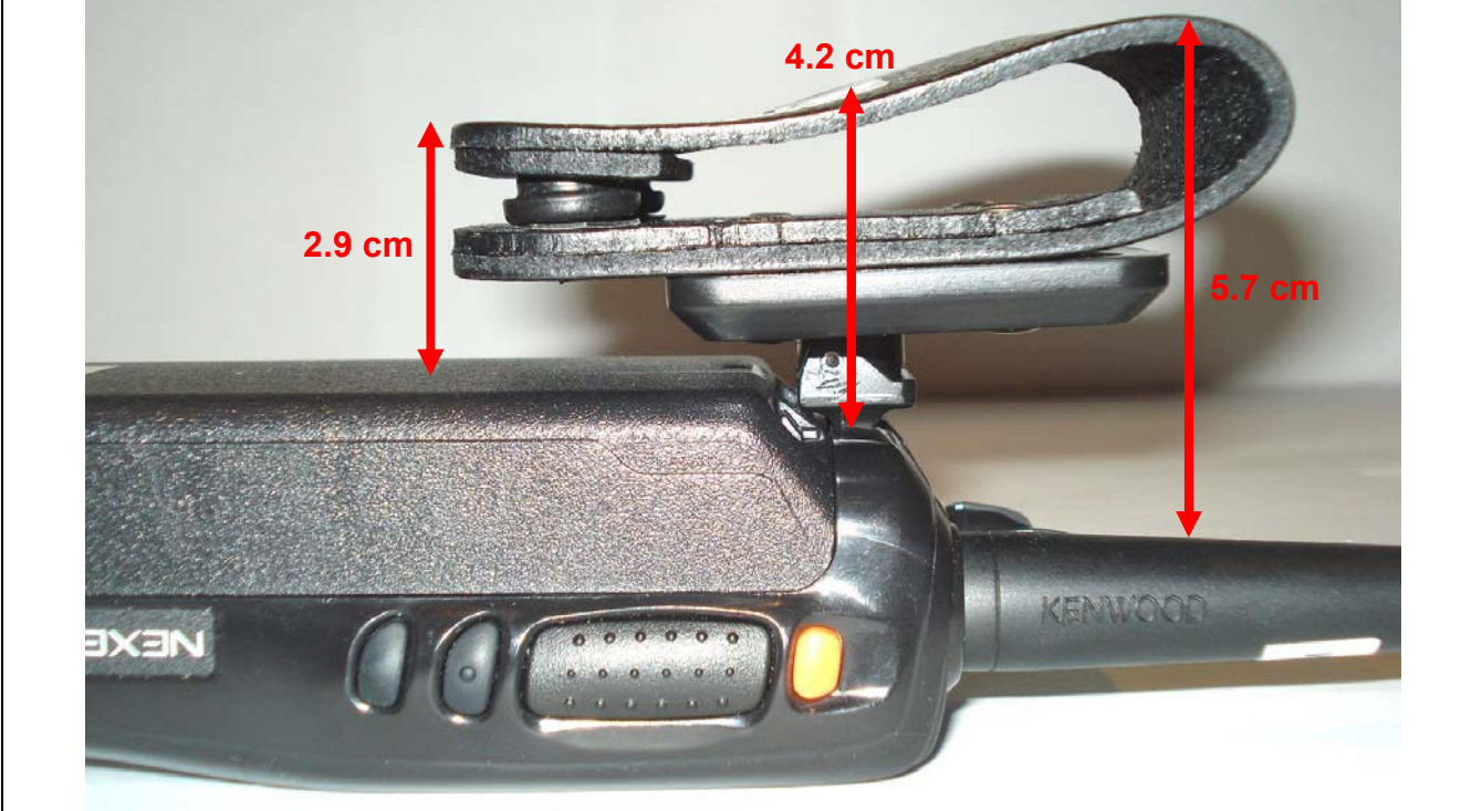
KBH-13DS Swivel Belt-Loop measurement distance from Back of DUT & Antenna Base – KBP-5 Alkaline Case “Battery d”
