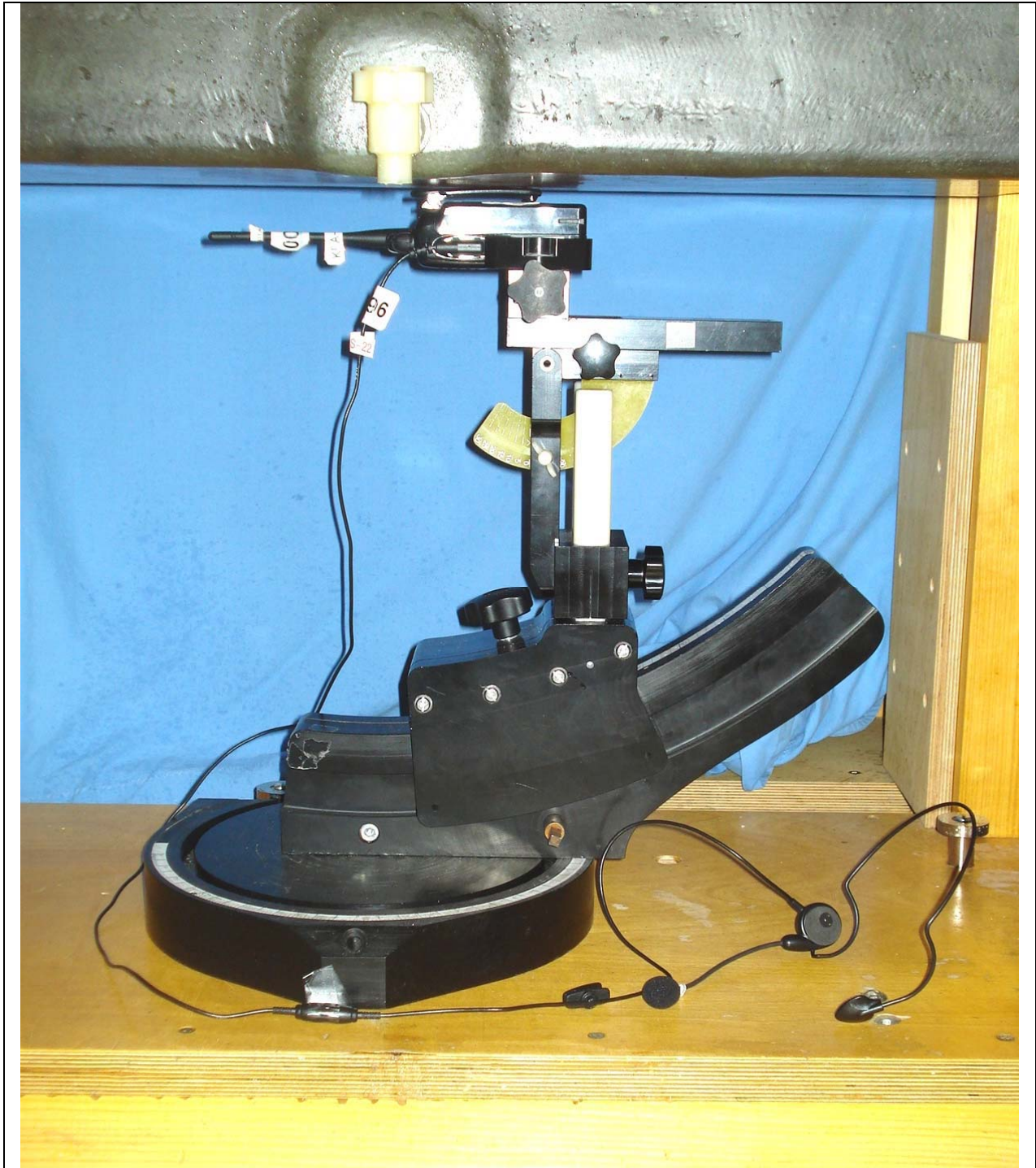
NX-320-K3 with Belt-Clip Body-worn Accessory (P/N: KBH-12) & Add. Audio Accessory - Category #1 - Headset (Behind-the-Head Headset w/ Boom-Mic & PTT P/N: KHS-22) (Battery Parallel to Planar Phantom)
