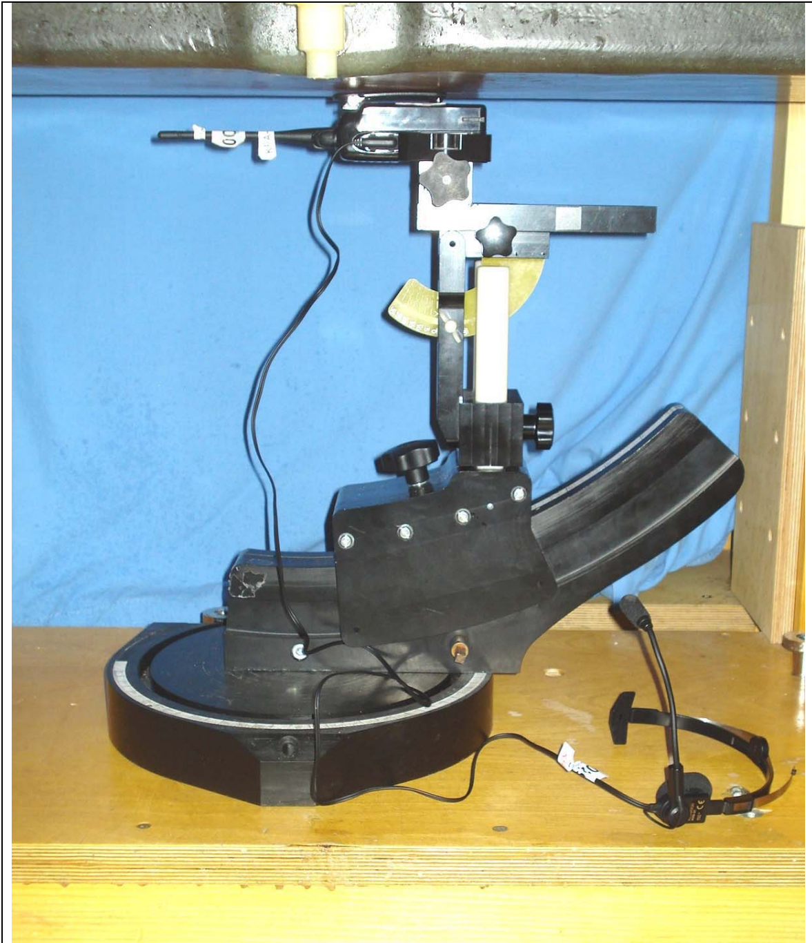
NX-320-K3 with Belt-Clip Body-worn Accessory (P/N: KBH-12) & Add. Audio Accessory - Category #1 - Headset (Lightweight Headset - no VOX or PTT controls P/N: KHS-21) (Battery Parallel to Planar Phantom)
