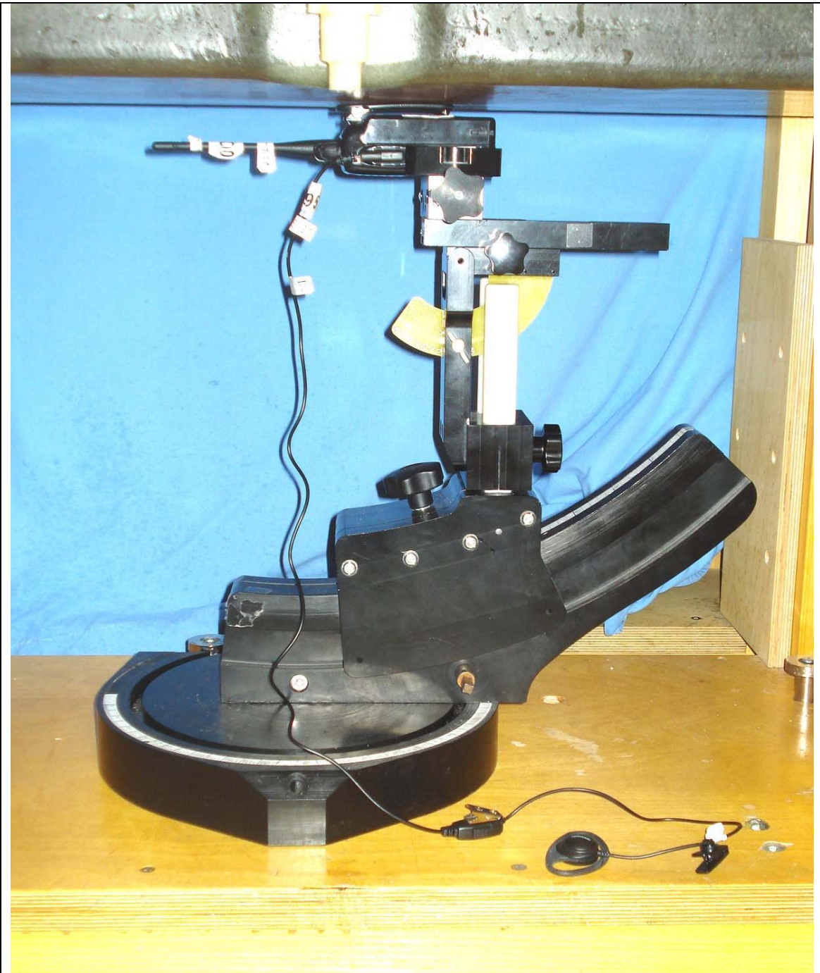
NX-320-K3 with Belt-Clip Body-worn Accessory (P/N: KBH-12) & Default Audio Accessory - Category #2 - Earpiece (D-Ring Ear Hanger w/ PTT & Mic P/N: KHS-27) (Battery Parallel to Planar Phantom)
