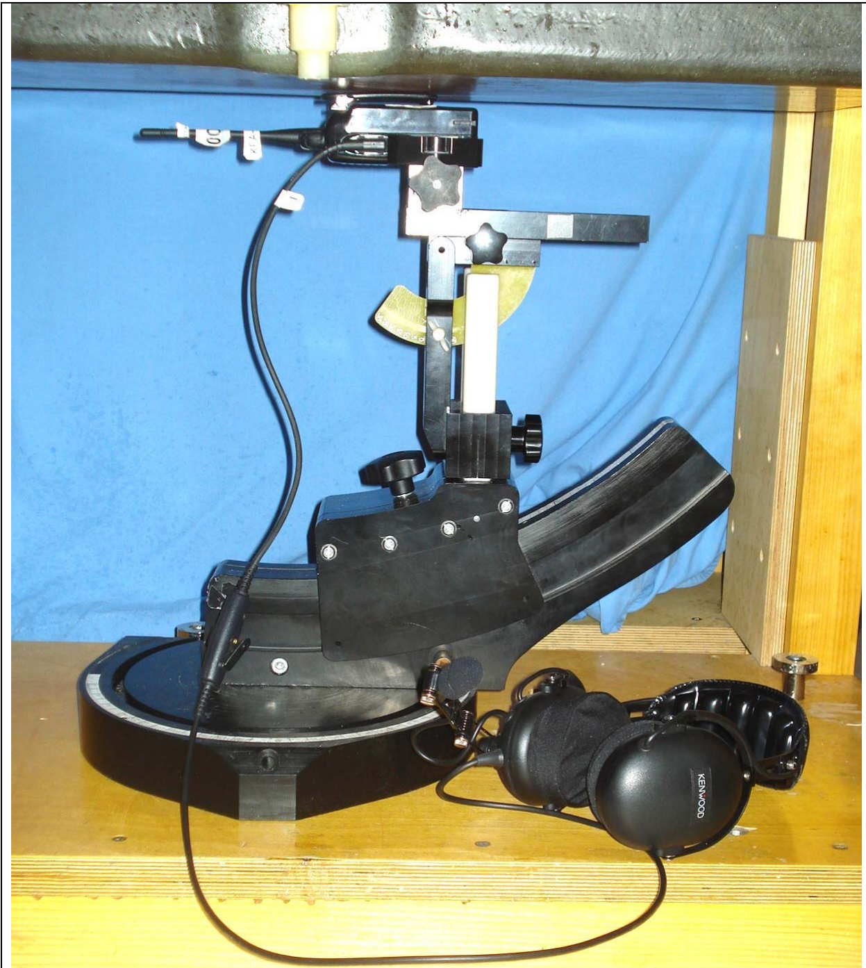
NX-320-K3 with Belt-Clip Body-worn Accessory (P/N: KBH-12) & Add. Audio Accessory - Category #1 - Headset (Noise Reduction Headset - Over-the-Head P/N: KHS-10-OH) (Battery Parallel to Planar Phantom)
