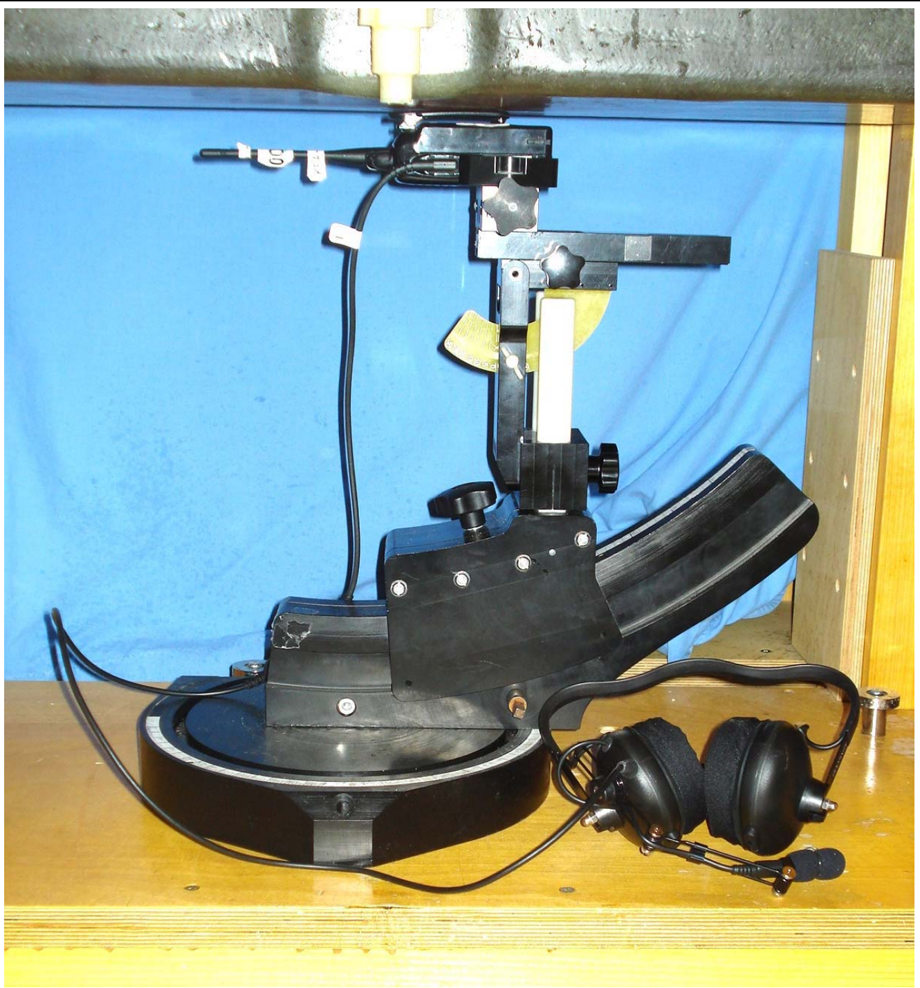
NX-320-K3 Body-worn SAR Test Setup with KBH-12 Belt-Clip and Default Audio Accessory (Headset P/N: KHS-10-BH) (Battery Parallel to Planar Phantom)
