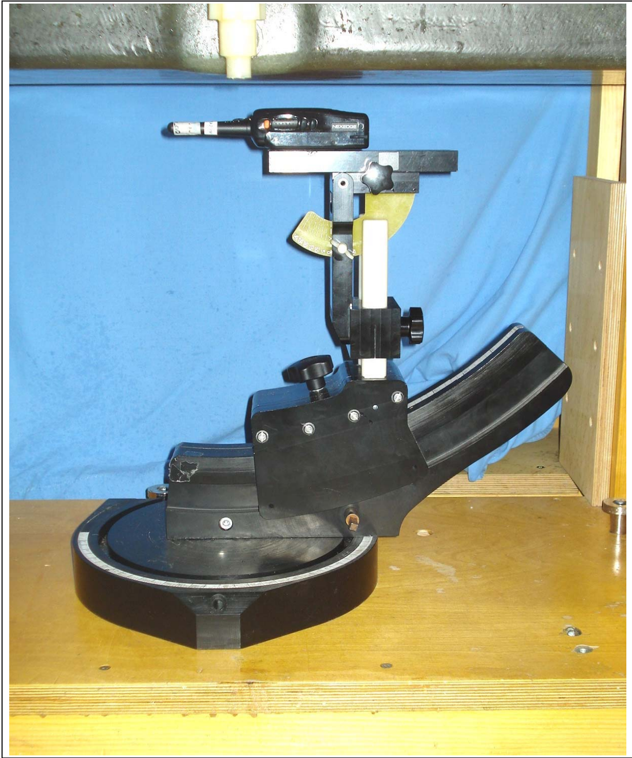
Face-held SAR Configuration Test Setup
