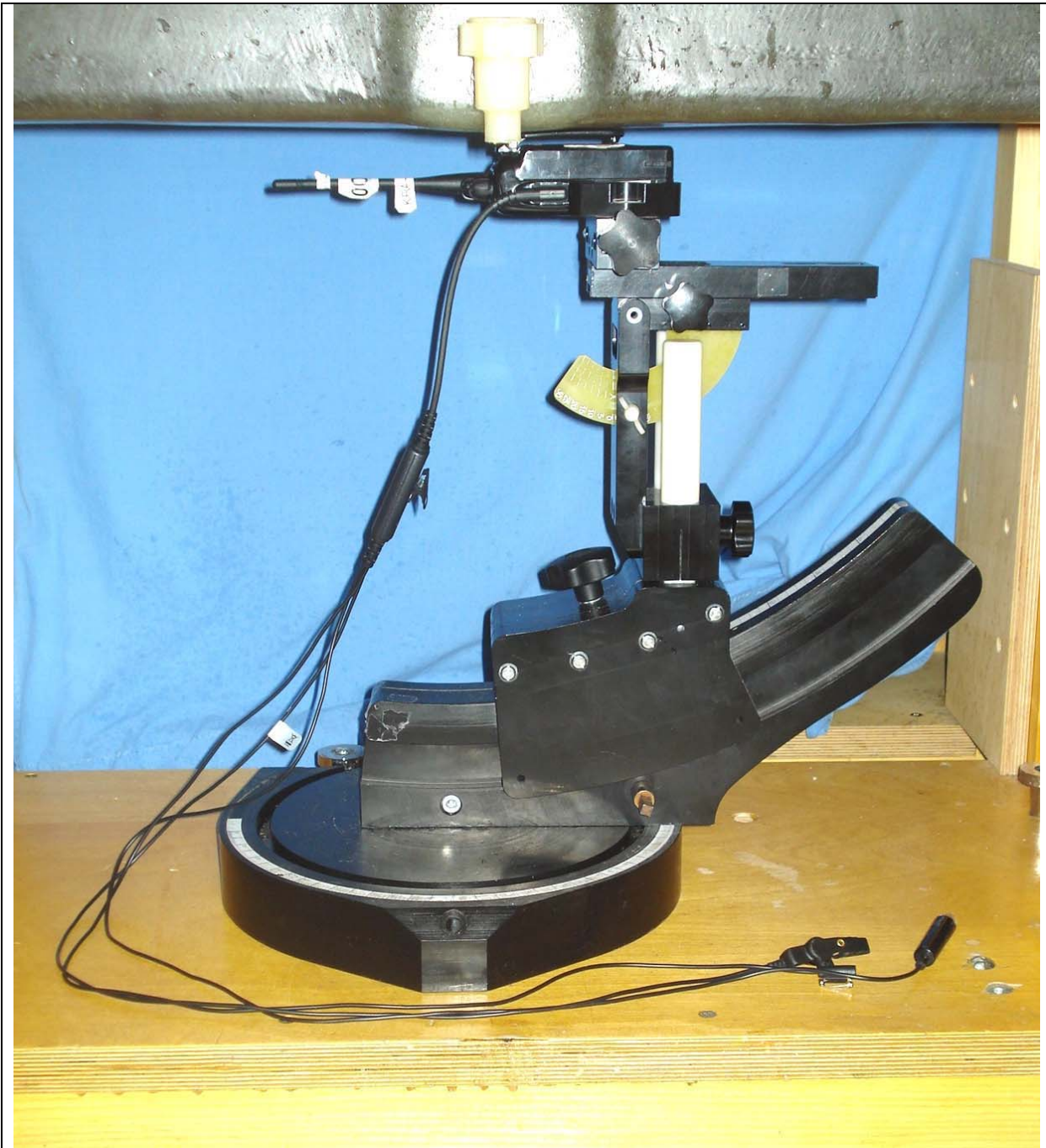
NX-320-K3 with Belt-Clip Body-worn Accessory (P/N: KBH-12) & Default Audio Accessory - Category #3 - Palm-Mic Kit (3-Wire Lapel Microphone w/ Earpiece P/N: KHS-9BL) (Battery Parallel to Planar Phantom)
