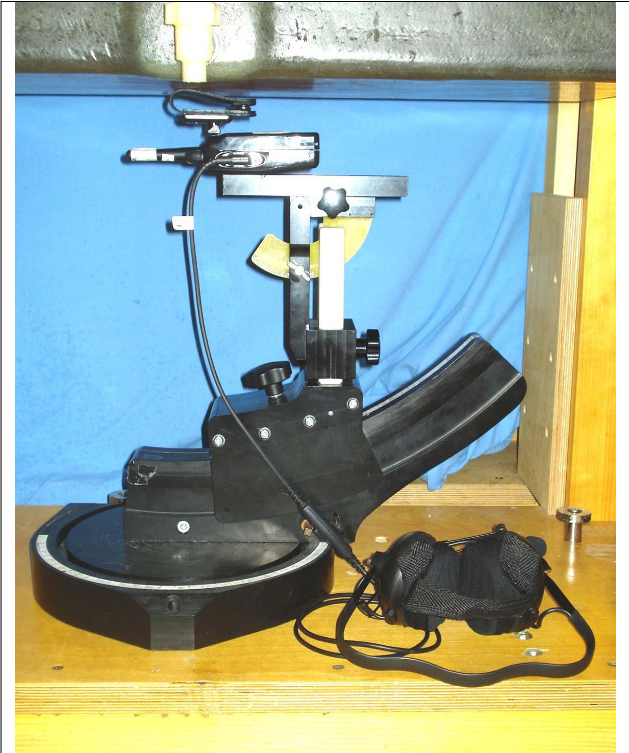
NX-320-K3 Body-worn SAR Test Setup w/ KBH-13DS Swivel Belt-Loop & Default Audio Accessory (Headset P/N: KHS-10-BH) (Battery Parallel to Planar Phantom)
