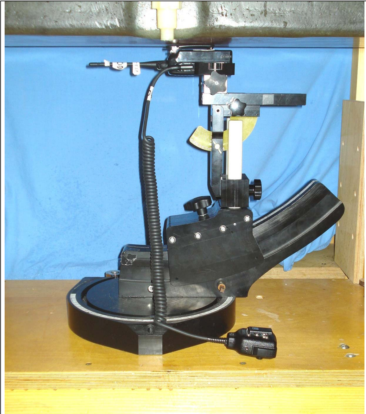
NX-320-K3 with Belt-Clip Body-worn Accessory (P/N: KBH-12) & Default Audio Accessory - Category #4 - Speaker-Microphone (Speaker-Mic w/ Integral GPS Unit P/N: KMC-48GPS) (Battery Parallel to Planar Phantom)
