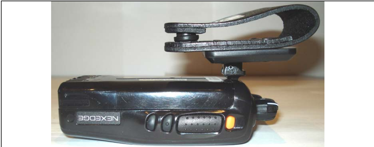
Left Side of DUT with KNB-55L Li-ion "Battery b" & Swivel Belt-Loop accessory
