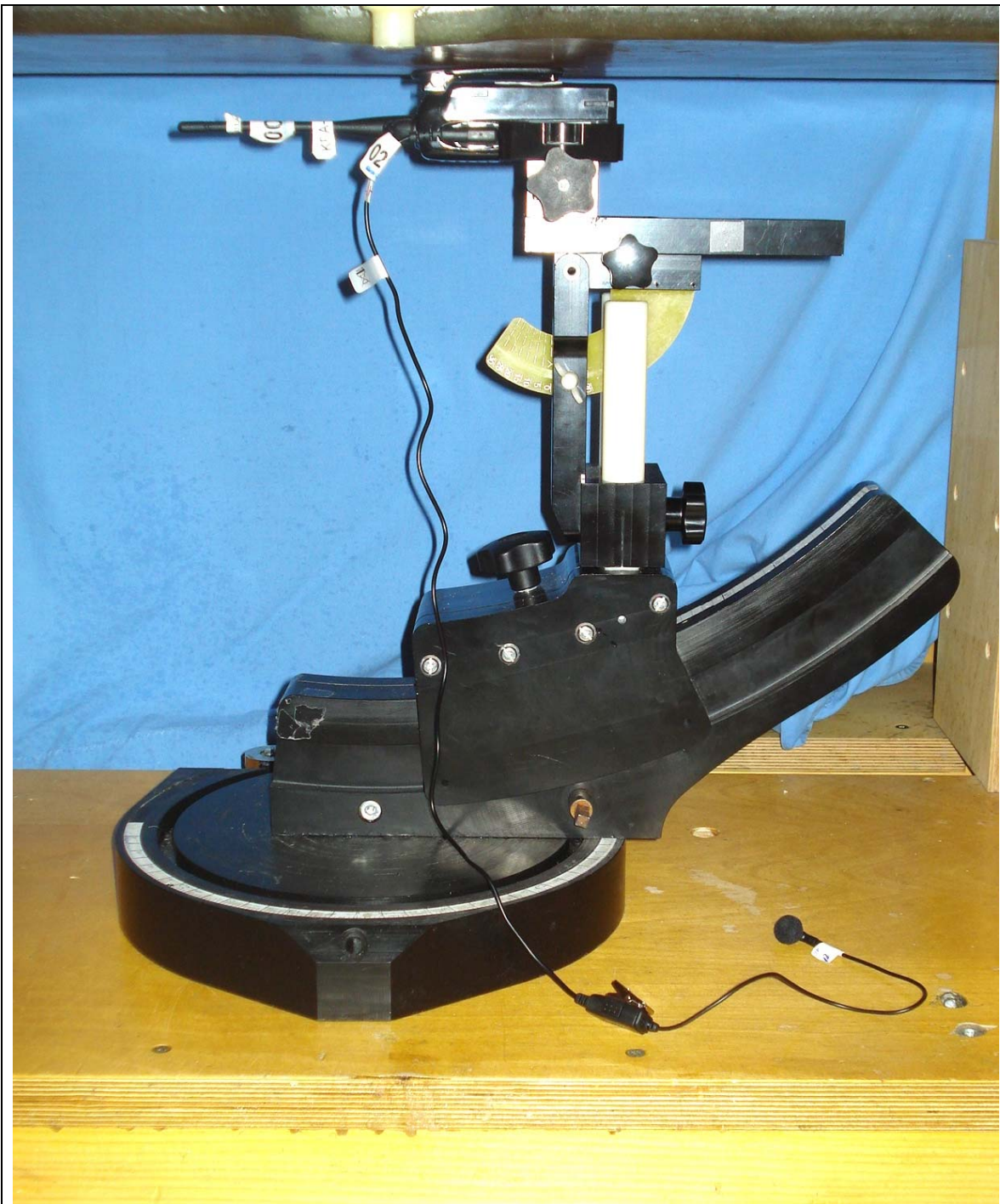
DUT with Belt-Clip Body-worn Accessory (P/N: KBH-12) & Add. Audio Accessory - Category #2 - Earpiece (Clip Mic w/ Earphone P/N: KHS-26) (Battery Parallel to Planar Phantom)
