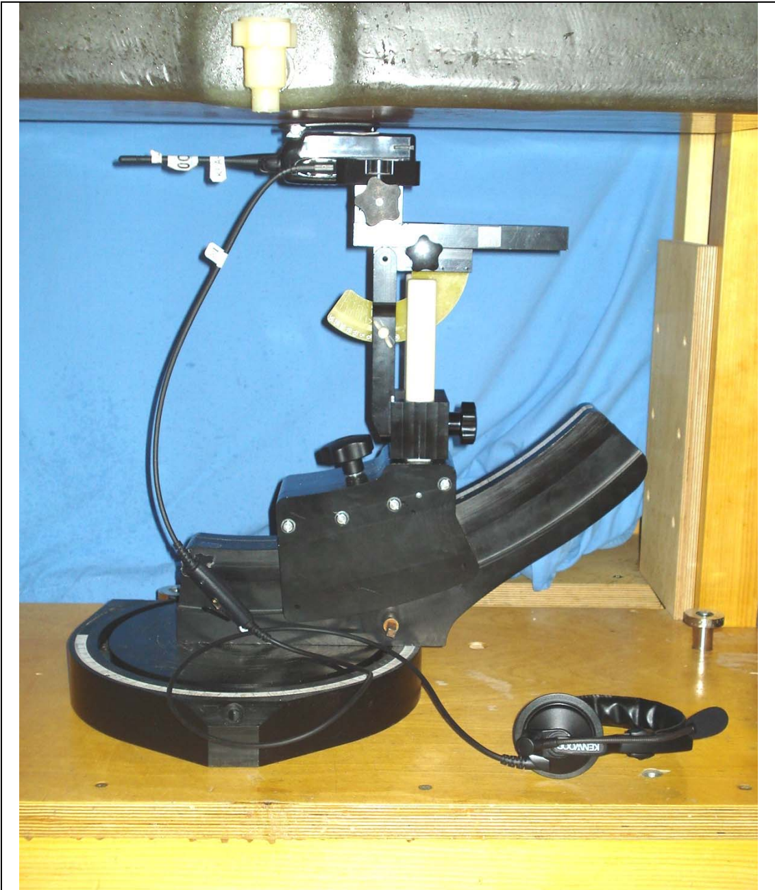
DUT with Belt-Clip Body-worn Accessory (P/N: KBH-12) & Add. Audio Accessory - Category #1 - Headset (Single Muff Headset w/ Boom-Mic & PTT P/N: KHS-7A) (Battery Parallel to Planar Phantom)
