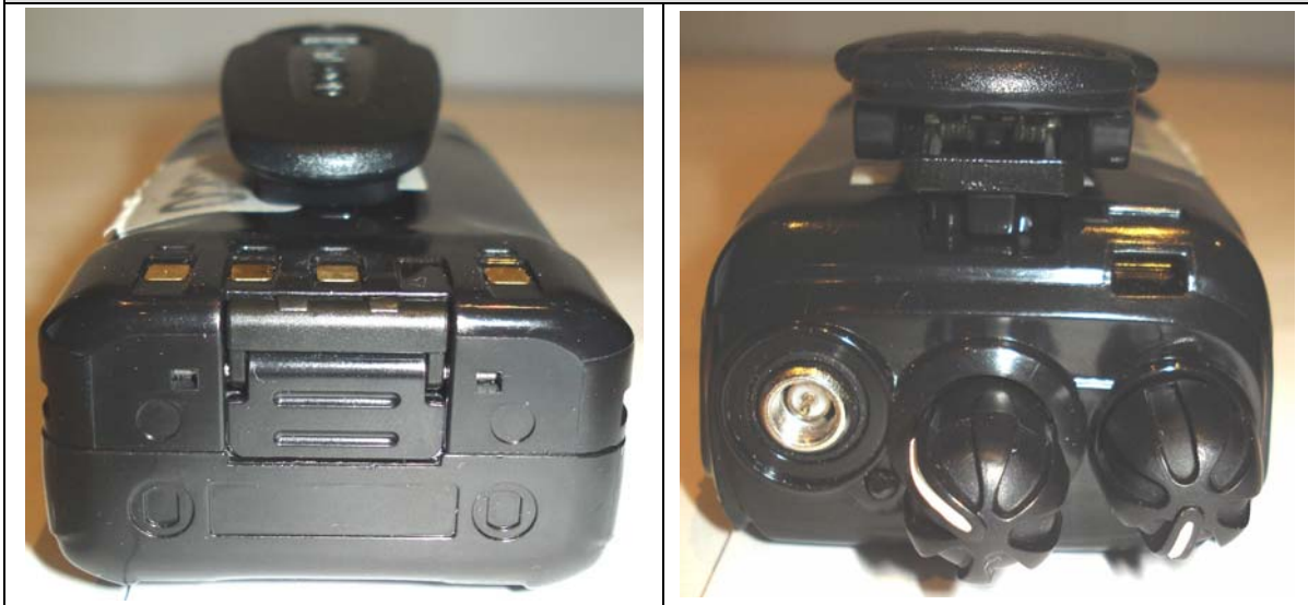
Bottom end of DUT with KNB-55L "Battery b" & Belt-Clip Top end of DUT with KNB-55L "Battery b" & Belt-Clip
