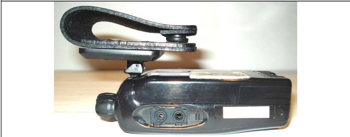
Right Side of DUT with KNB-57L Li-ion "Battery a" & Swivel Belt-Loop accessory
