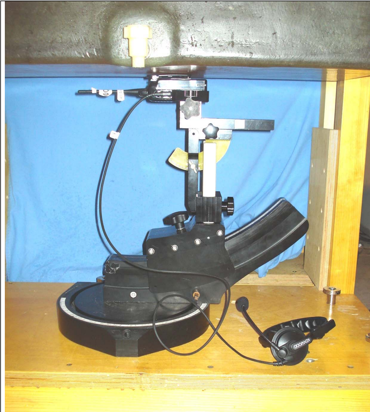
DUT with Belt-Clip Body-worn Accessory (P/N: KBH-12) & Add. Audio Accessory - Category #1 - Headset (Single Muff Headset w/ Boom-Mic P/N: KHS-7) (Battery Parallel to Planar Phantom)
