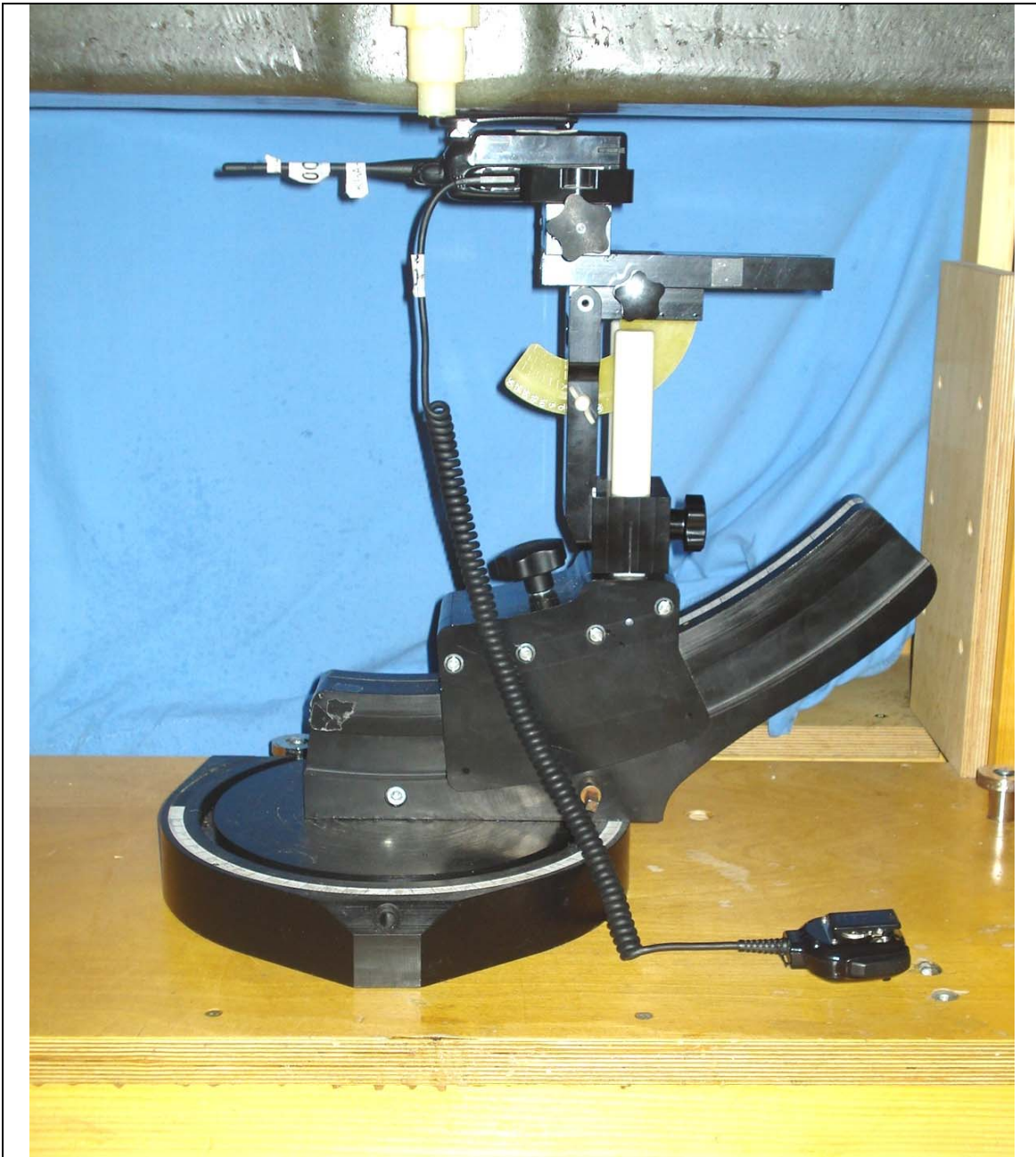
DUT with Belt-Clip Body-worn Accessory (P/N: KBH-12) & Add. Audio Accessory - Category #4 - Speaker-Microphone (Heavy-Duty Speaker-Mic P/N: KMC-45) (Battery Parallel to Planar Phantom)
