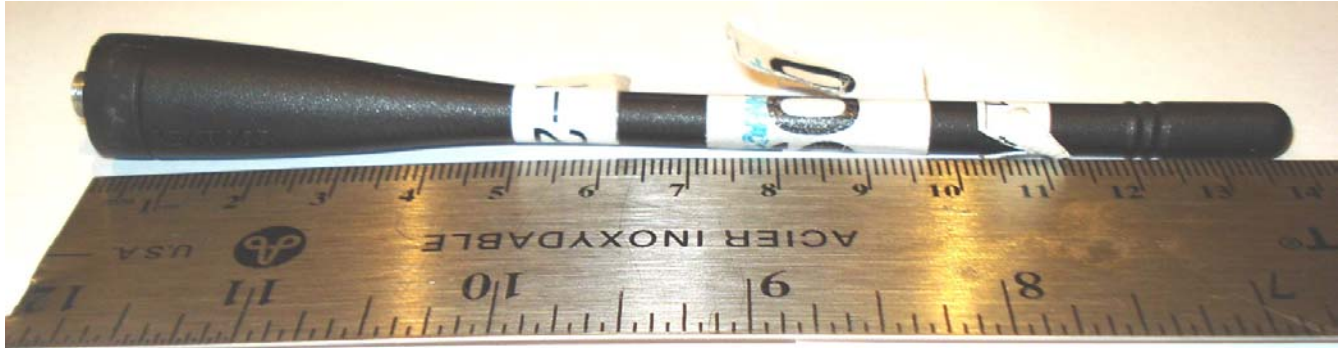
Detachable Whip "Antenna D" P/N: KRA-27M2 (Length = 139 mm)
