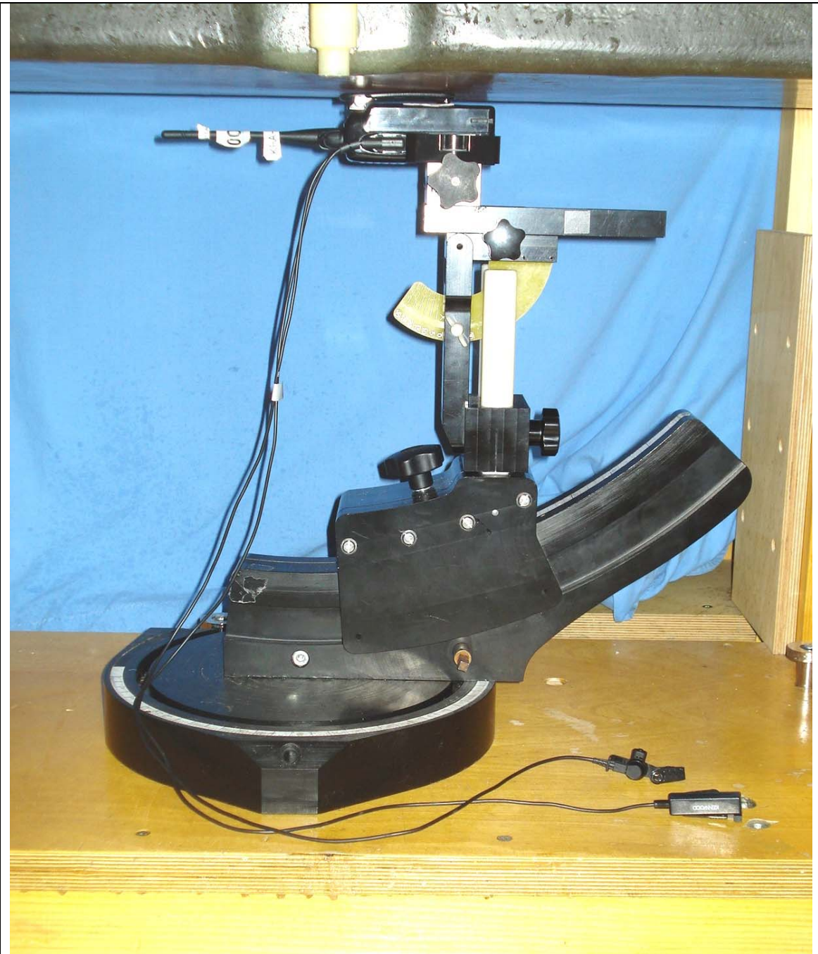
DUT with Belt-Clip Body-worn Accessory (P/N: KBH-12) & Add. Audio Accessory - Category #3 - Palm-Mic Kit (2-Wire Palm-Mic w/ Earphone P/N: KHS-8BL) (Battery Parallel to Planar Phantom)
