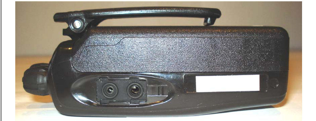
Right Side of DUT with KBP-5 Alkaline Case "Battery d" & Belt-Clip accessory
