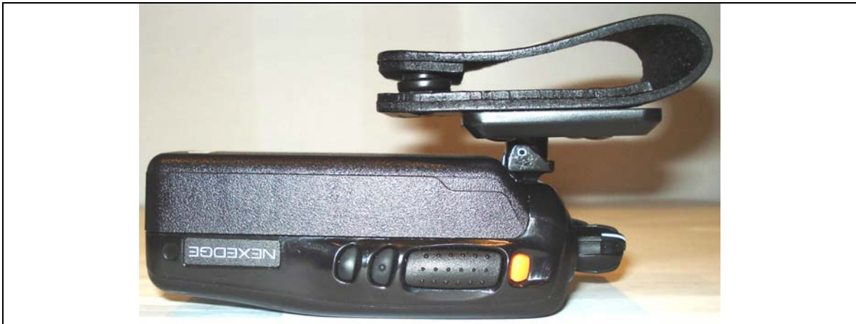
Left Side of DUT with KBP-5 Alkaline Case "Battery d" & Swivel Belt-Loop accessory
