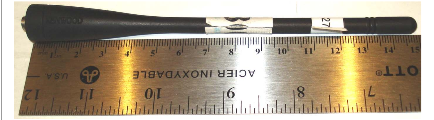
Detachable Whip "Antenna C" P/N: KRA-27M (Length = 149 mm)
