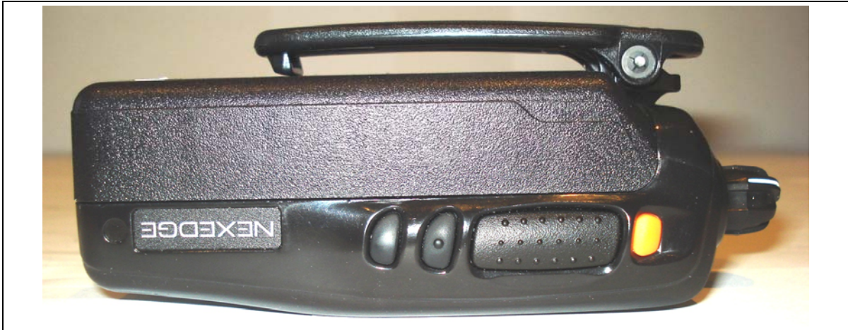
Left Side of DUT with KBP-5 Alkaline Case "Battery d" & Belt-Clip accessory
