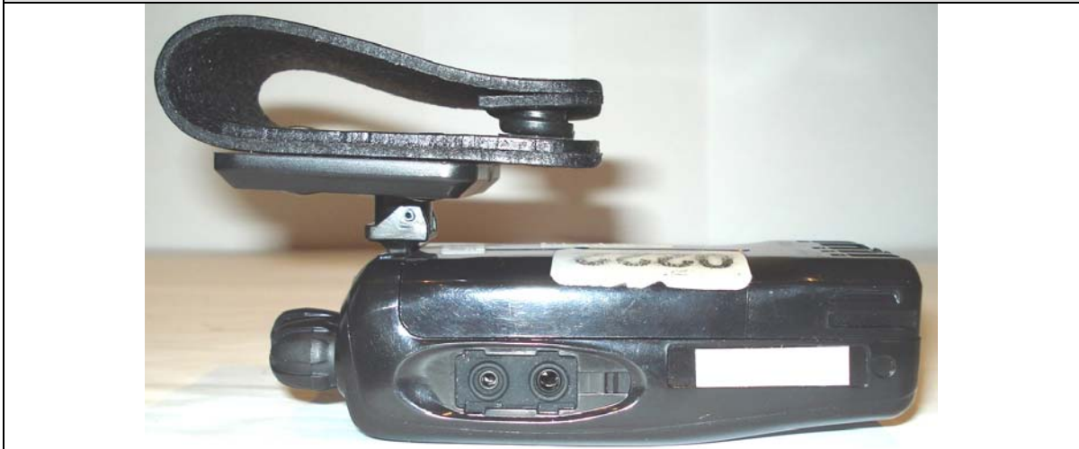
Right Side of DUT with KNB-55L Li-ion "Battery b" & Swivel Belt-Loop accessory
