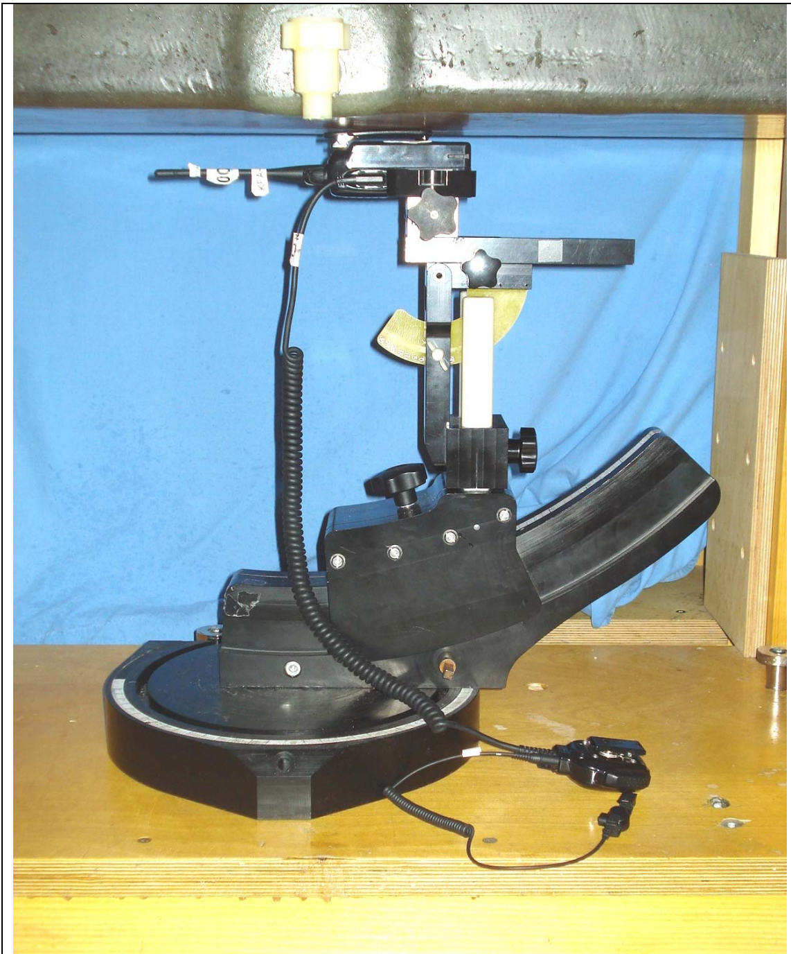
DUT with Belt-Clip Body-worn Accessory (P/N: KBH-12) & Add. Audio Accessory - Category #4 - Speaker-Microphone (Heavy-Duty Speaker-Mic P/N: KMC-45 with Earphone Kit P/N: KEP-2) (Battery Parallel to Planar Phantom)
