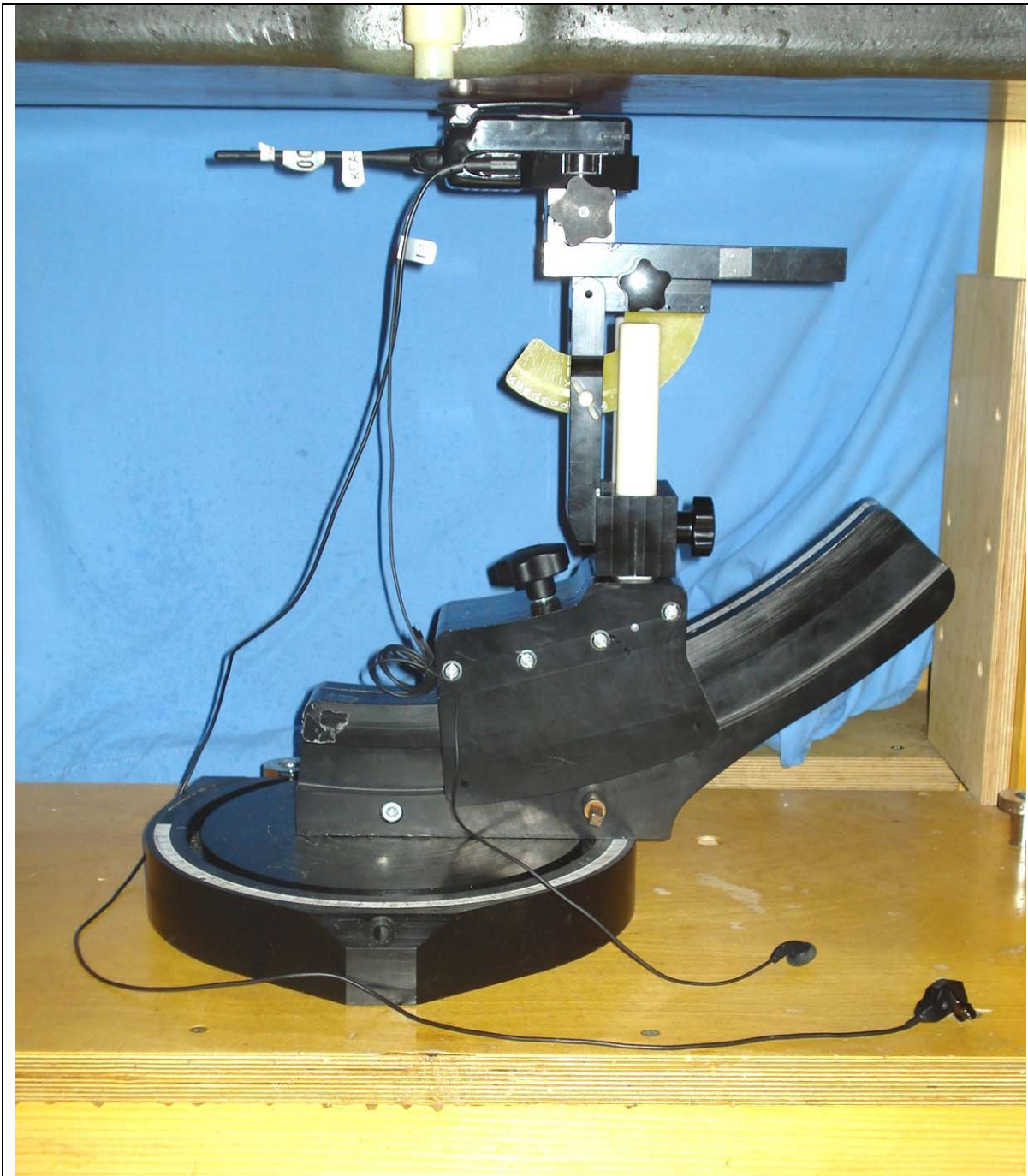
DUT with Belt-Clip Body-worn Accessory (P/N: KBH-12) & Add. Audio Accessory - Category #2 - Earpiece (2-Wire Ear-Bud w/ mic/PTT - Vox Ready P/N: KHS-23) (Battery Parallel to Planar Phantom)
