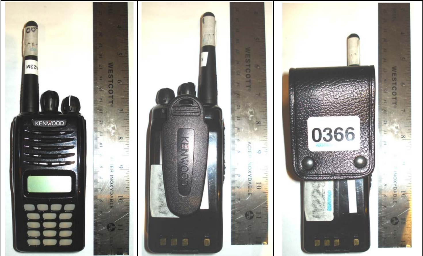
Front of DUT with KRA-23M Antenna Back of DUT with KRA-23M & Belt-Clip Back of DUT with KRA-23M & Swivel Belt-Loop
