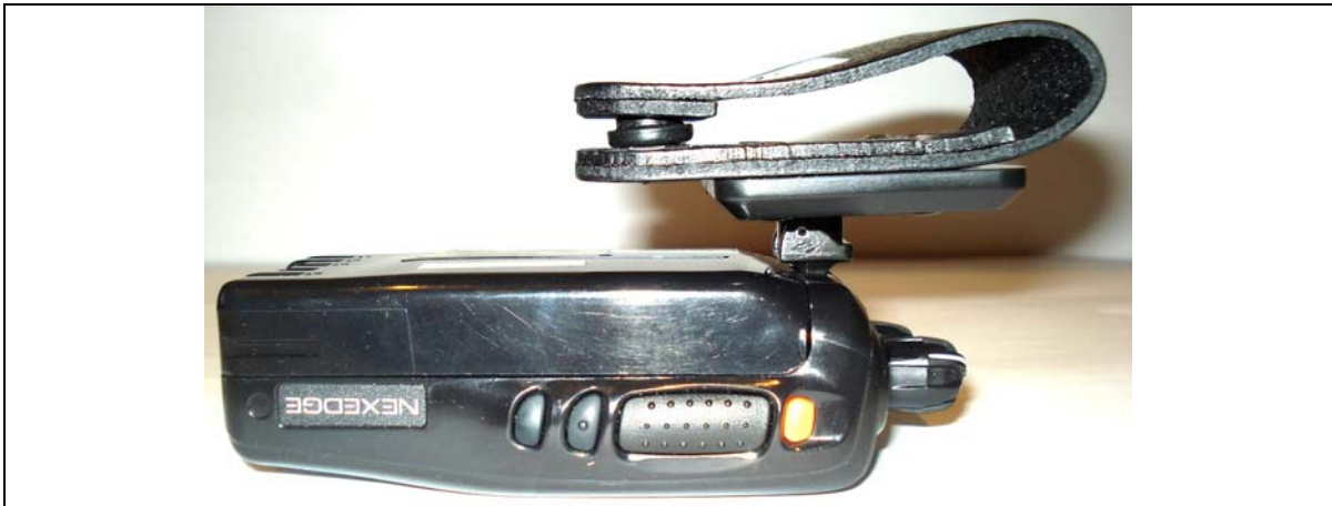
Left Side of DUT with KNB-57L Li-ion "Battery a" & Swivel Belt-Loop accessory
