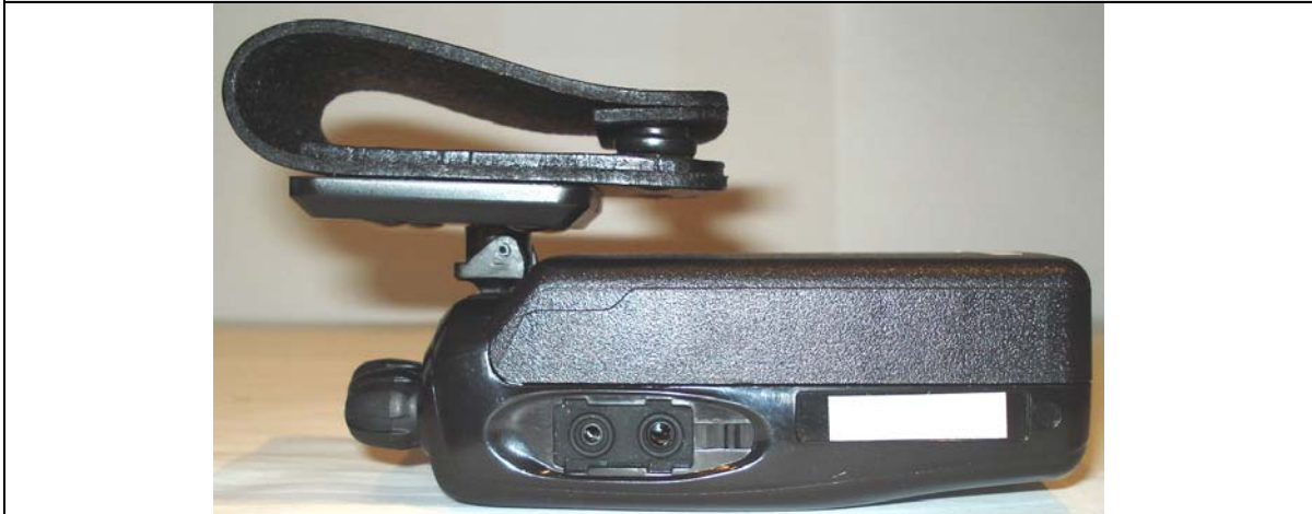
Right Side of DUT with KBP-5 Alkaline Case "Battery d" & Swivel Belt-Loop accessory
