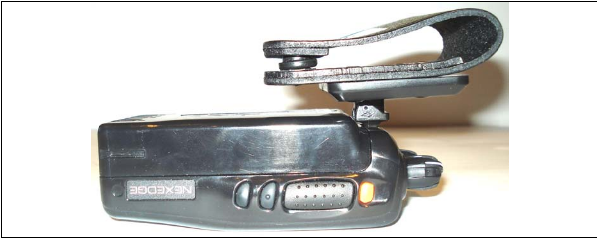
Left Side of DUT with KNB-56N Ni-MH "Battery c" & Swivel Belt-Loop accessory
