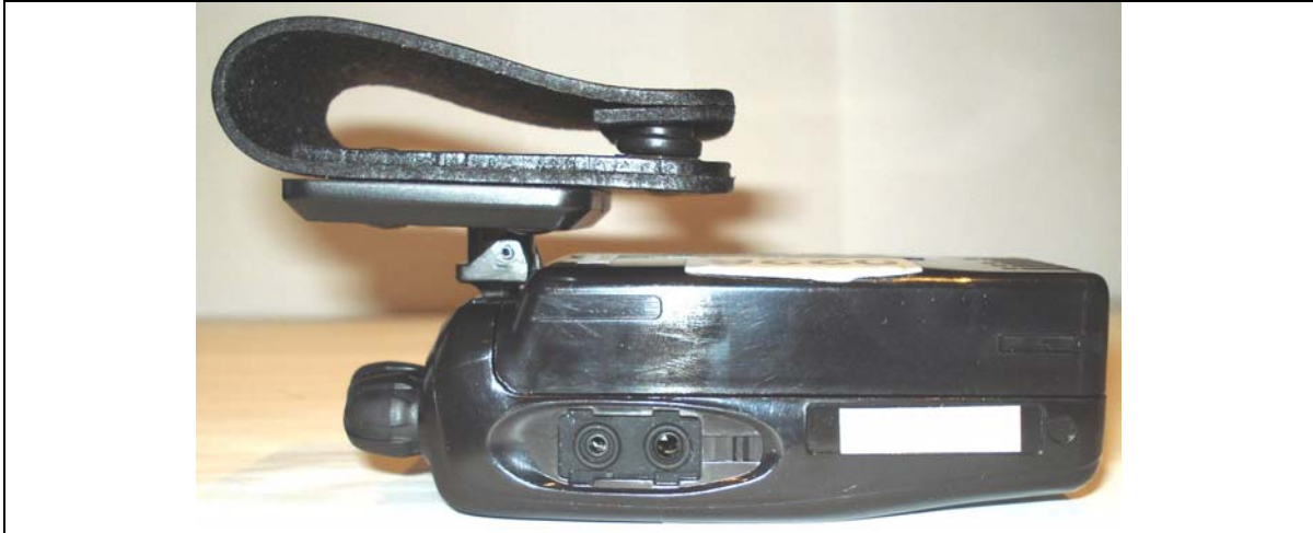
Right Side of DUT with KNB-56N Ni-MH "Battery c" & Swivel Belt-Loop accessory
