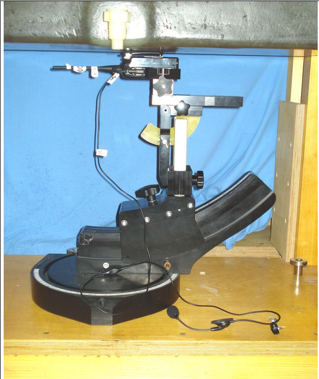
DUT with Belt-Clip Body-worn Accessory (P/N: KBH-12) & Add. Audio Accessory - Category #2 - Earpiece (Earhook w/ Mini Boom-Mic P/N: KHS-25) (Battery Parallel to Planar Phantom)
