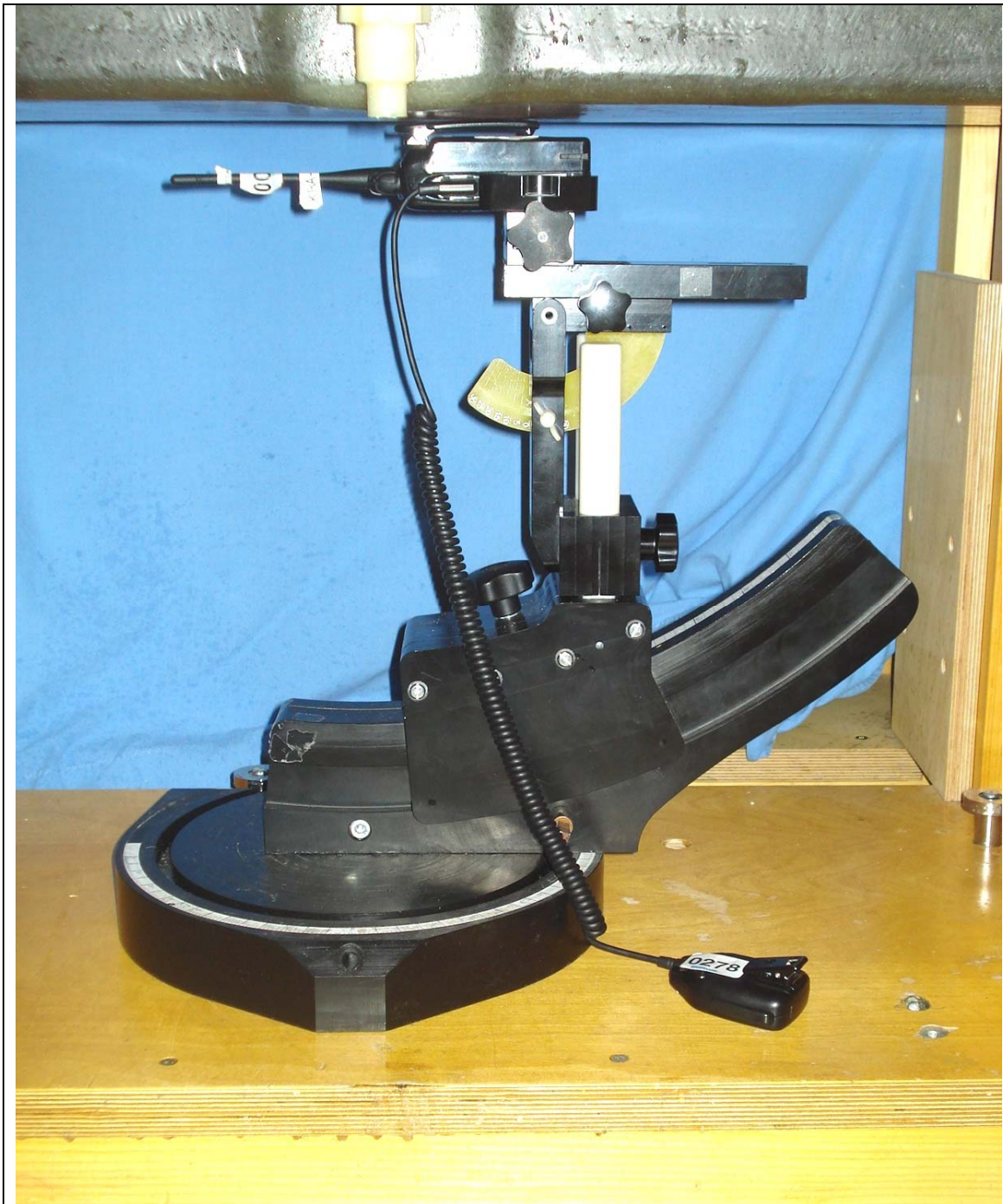
DUT with Belt-Clip Body-worn Accessory (P/N: KBH-12) & Add. Audio Accessory - Category #4 - Speaker-Microphone (Slim-Line Speaker-Mic P/N: KMC-21) (Battery Parallel to Planar Phantom)
