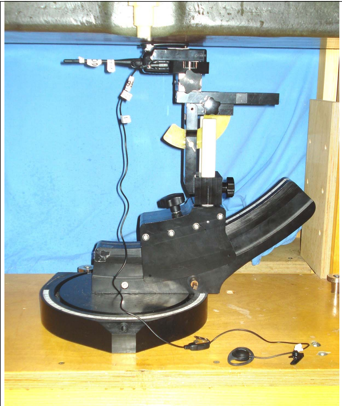
DUT with Belt-Clip Body-worn Accessory (P/N: KBH-12) & Default Audio Accessory - Category #2 - Earpiece (D-Ring Ear Hanger w/ PTT & Mic P/N: KHS-27) (Battery Parallel to Planar Phantom)
