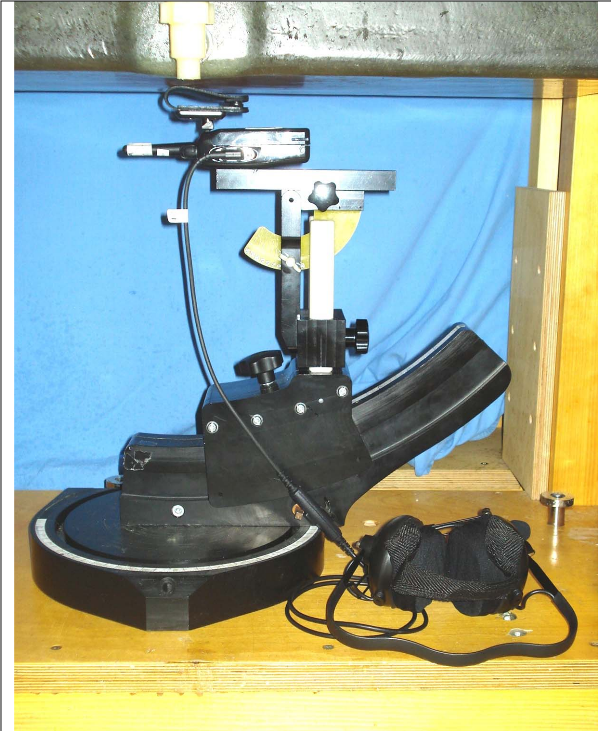
Body-worn SAR Test Setup with KBH-13DS Swivel Belt-Loop and Default Audio Accessory (Headset P/N: KHS-10-BH) (Battery Parallel to Planar Phantom)
