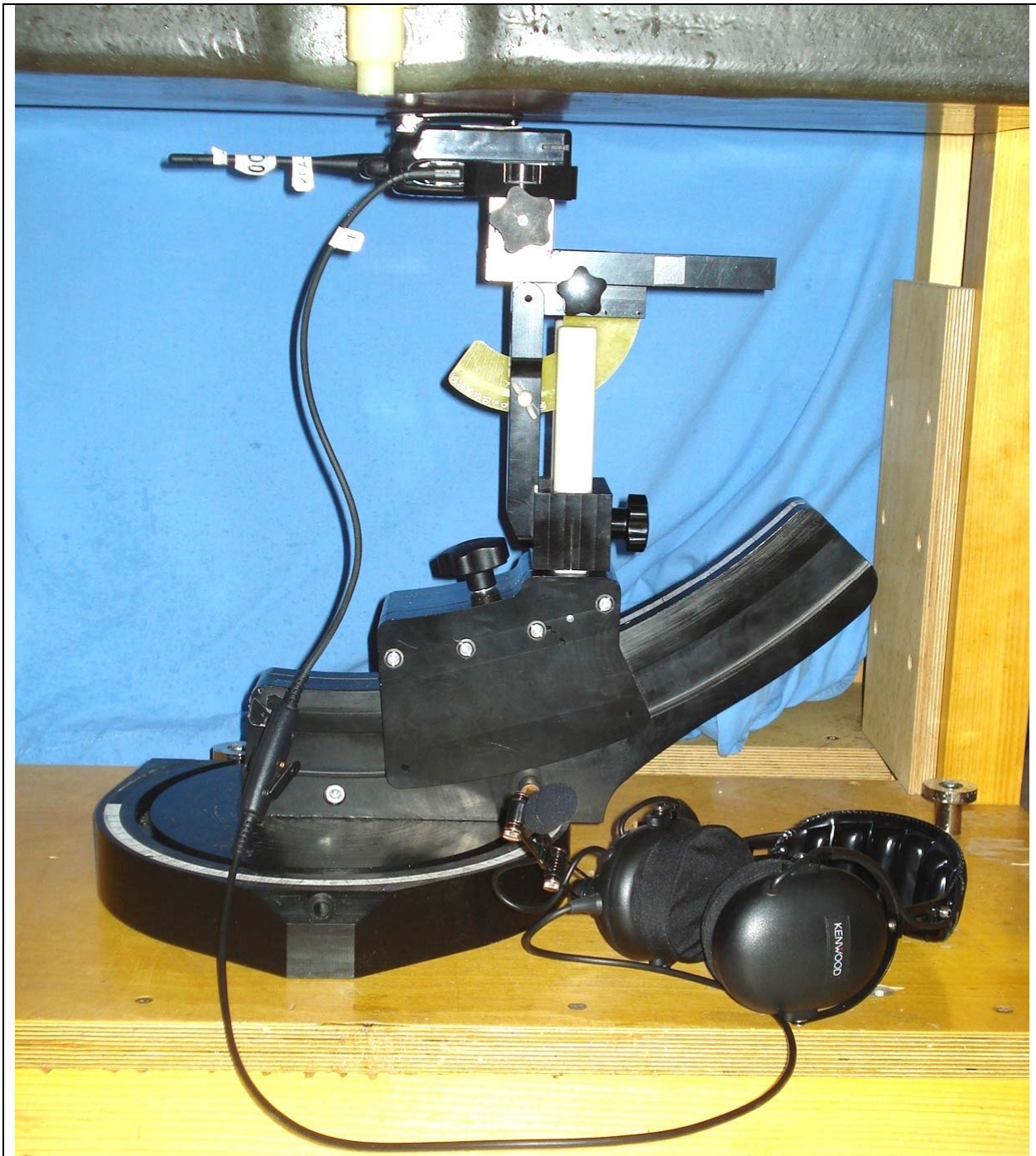
DUT with Belt-Clip Body-worn Accessory (P/N: KBH-12) & Add. Audio Accessory - Category #1 - Headset (Noise Reduction Headset - Over-the-Head P/N: KHS-10-OH) (Battery Parallel to Planar Phantom)
