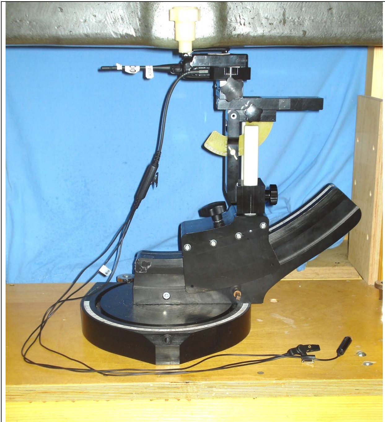
DUT with Belt-Clip Body-worn Accessory (P/N: KBH-12) & Default Audio Accessory - Category #3 - Palm-Mic Kit (3-Wire Lapel Microphone w/ Earpiece P/N: KHS-9BL) (Battery Parallel to Planar Phantom)
