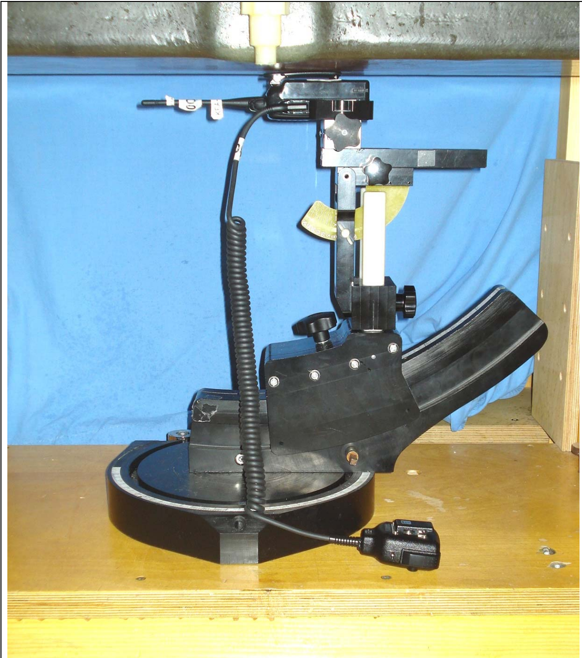
DUT with Belt-Clip Body-worn Accessory (P/N: KBH-12) & Default Audio Accessory - Category #4 - Speaker-Microphone (Speaker-Mic w/ Integral GPS Unit P/N: KMC-48GPS) (Battery Parallel to Planar Phantom)
