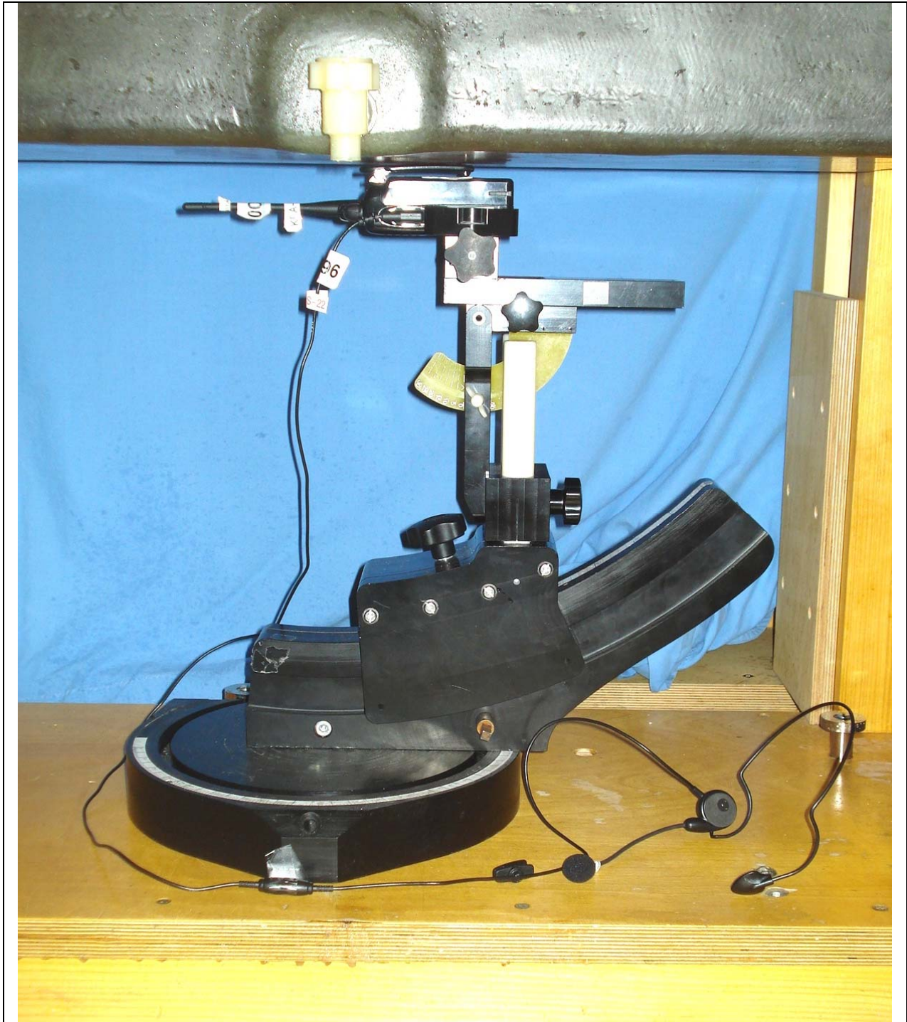
DUT with Belt-Clip Body-worn Accessory (P/N: KBH-12) & Add. Audio Accessory - Category #1 - Headset (Behind-the-Head Headset w/ Boom-Mic & PTT P/N: KHS-22) (Battery Parallel to Planar Phantom)
