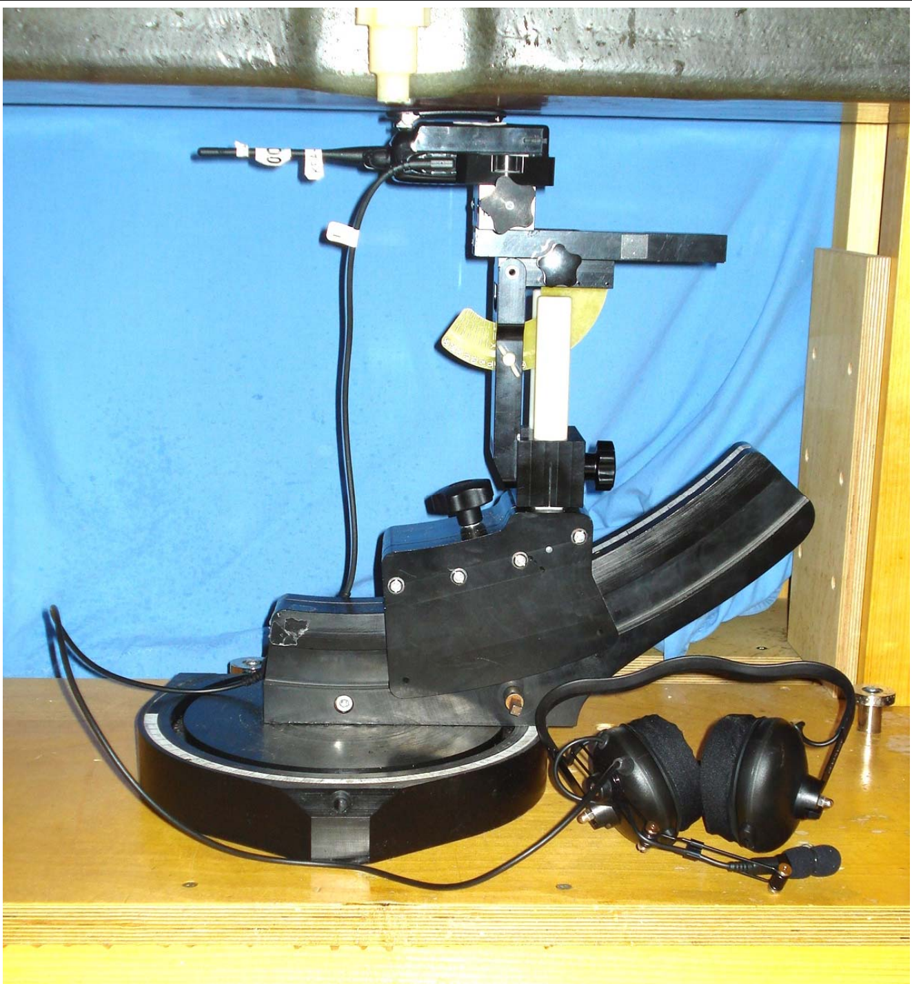
Body-worn SAR Test Setup with KBH-12 Belt-Clip and Default Audio Accessory (Headset P/N: KHS-10-BH) (Battery Parallel to Planar Phantom)
