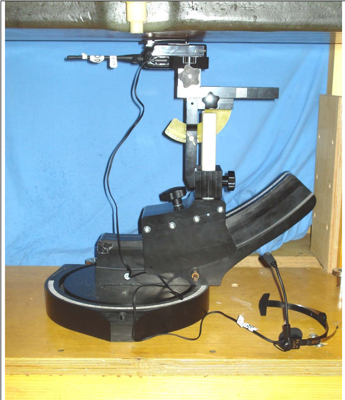
DUT with Belt-Clip Body-worn Accessory (P/N: KBH-12) & Add. Audio Accessory - Category #1 - Headset (Lightweight Headset - no VOX or PTT controls P/N: KHS-21) (Battery Parallel to Planar Phantom)
