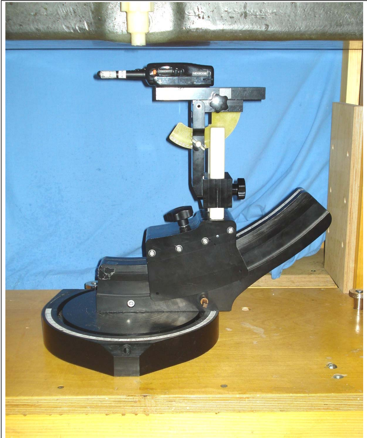
Face-held SAR Configuration Test Setup
