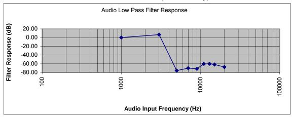
This unit is a digital radio and the roll-off for the filter is very linear in the operational band and sharp out of the band
