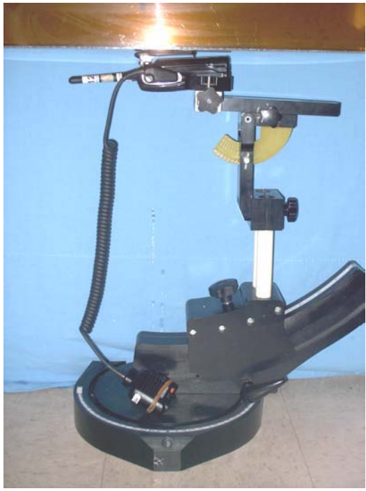
DUT with Ni-Cd/Ni-MH Battery (same dimensions), Stubby Antenna (P/N: KRA-22M) and KBH-10 Belt-Clip
