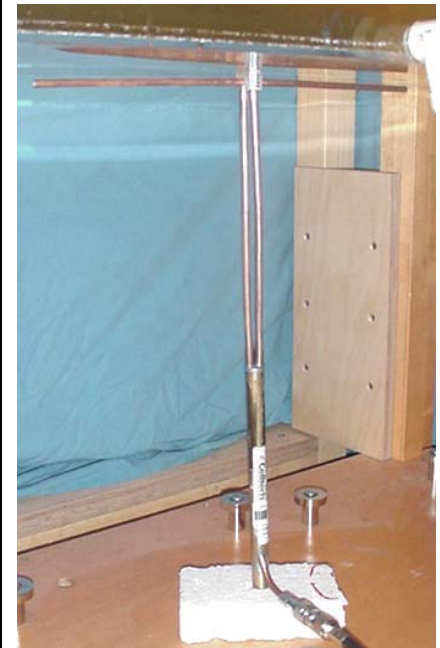
300 MHz Validation Dipole Setup
