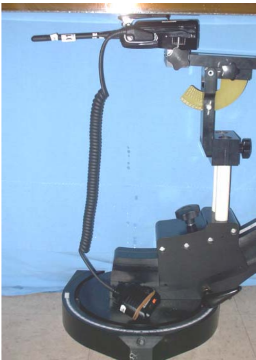
DUT with Ni-Cd/Ni-MH Battery (same dimensions), Whip Antenna (P/N: KRA-26M) and KBH-10 Belt-Clip
