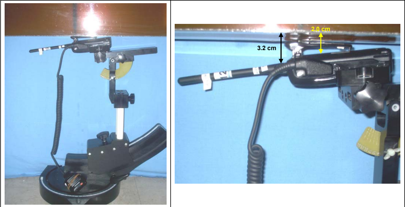
DUT with Li-ion Battery, Whip Antenna (P/N: KRA-26M) and KBH-11 Belt-Clip
