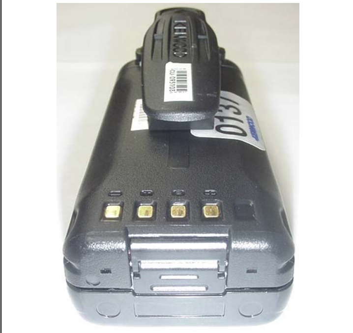
Bottom end of DUT with Lithium-ion Battery & KBH-10 Belt-Clip
