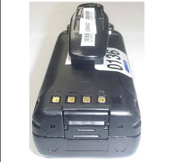
Bottom end of DUT with Lithium-ion Battery & KBH-11 Belt-Clip
